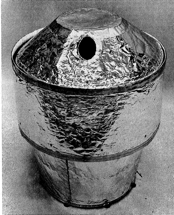
Figure 37. Apogee Motor Insulation
