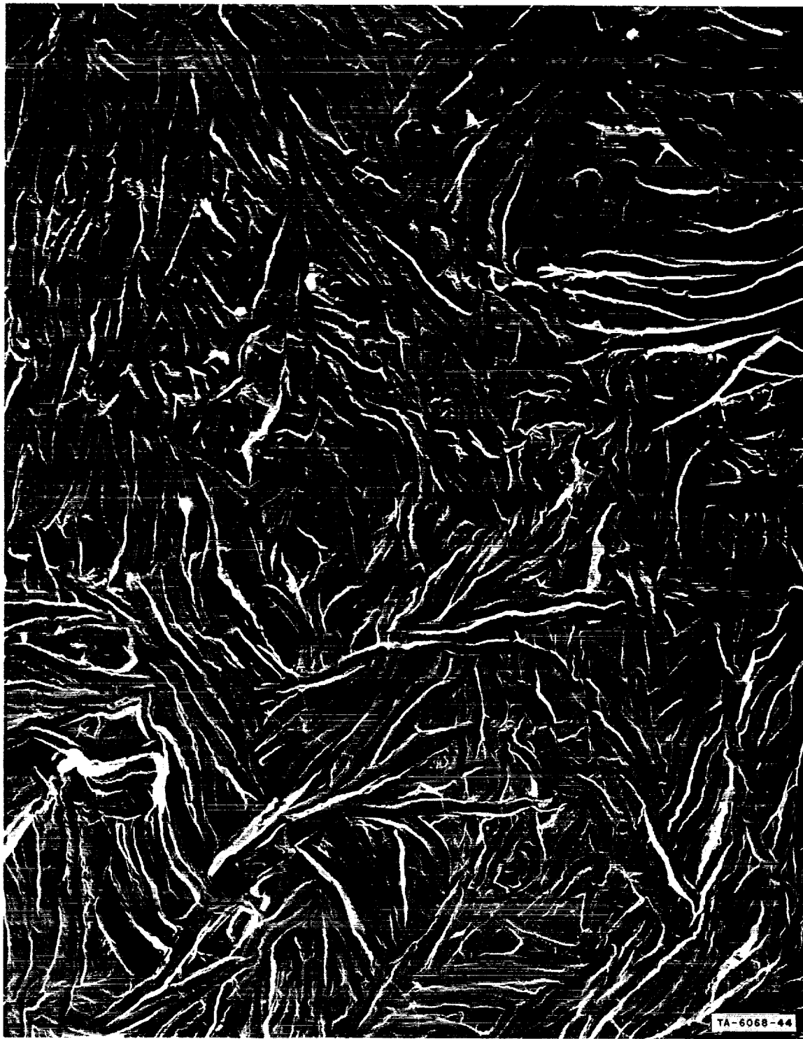
FIG. 13 ELECTRONMICROGRAPH OF TEFLON-TFE FILM SINTERED AT 350-370°C FOR 72 HOURS AND COOLED AT 2°C/MIN (8,000X)
