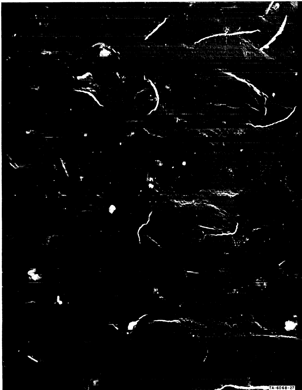
FIG. 12 ELECTRONMICROGRAPH (Direct Image) OF TEFLON-TFE FILM SINTERED 24 HOURS AT 370°C (8,000X)
