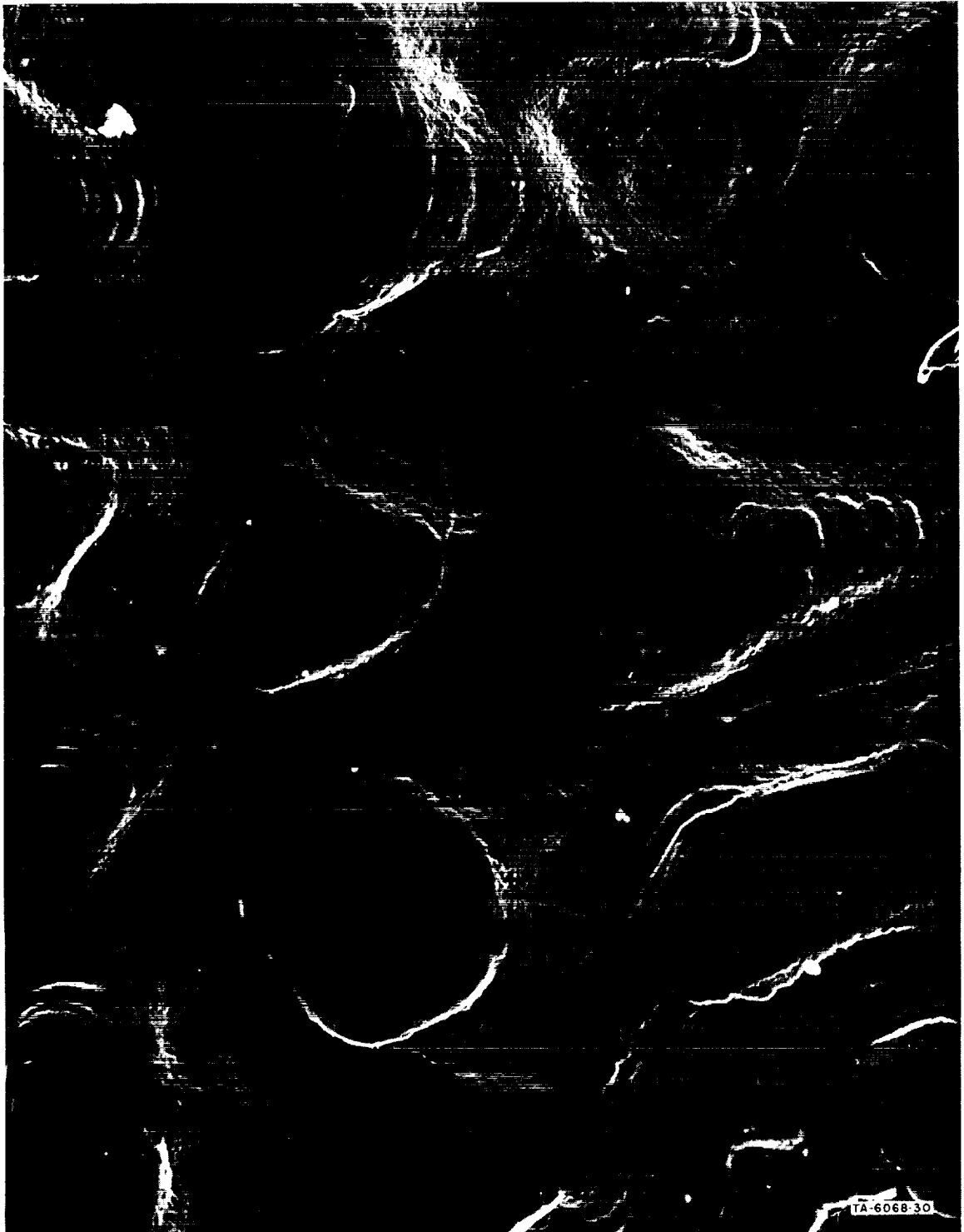
FIG. 10 ELECTRONMICROGRAPH (Direct Image) OF TEFLON-TFE FILM SINTERED 6 HOURS AT 370°C (8,000X)
