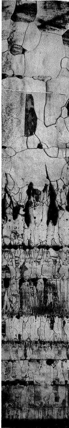
Figure V-7. Cross section of sample WC6B1 after 1 hour at 2000 °C.
