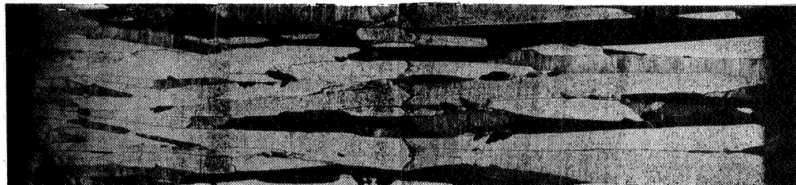
Figure V-4. Cross section of sample WF4D' after 100 hours at 1800°C.
