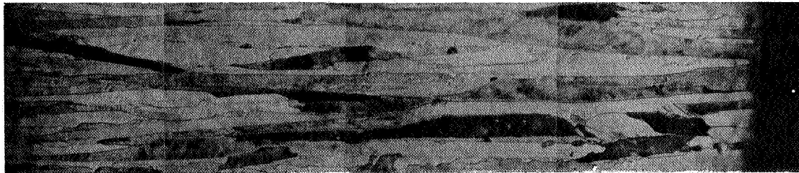
Figure V-3. Cross section of sample WF4C' after 30 hours at 1800°C.
