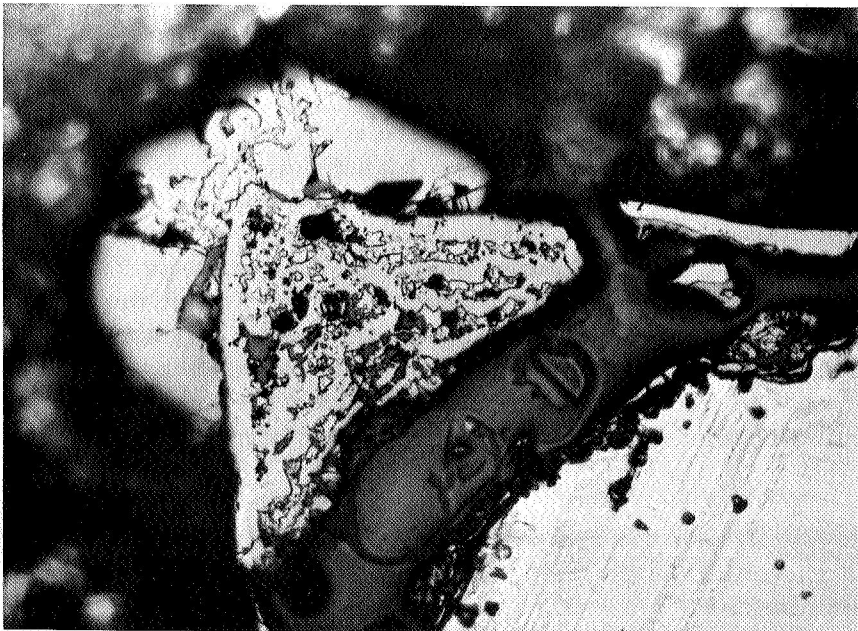
FIGURE 16. METALLOGRAPHIC CROSS SECTION OF Co-25Cr ALLOY OXIDIZED FOR 5.5 HOURS AT 1300 C AND 10 TORR OXYGEN
