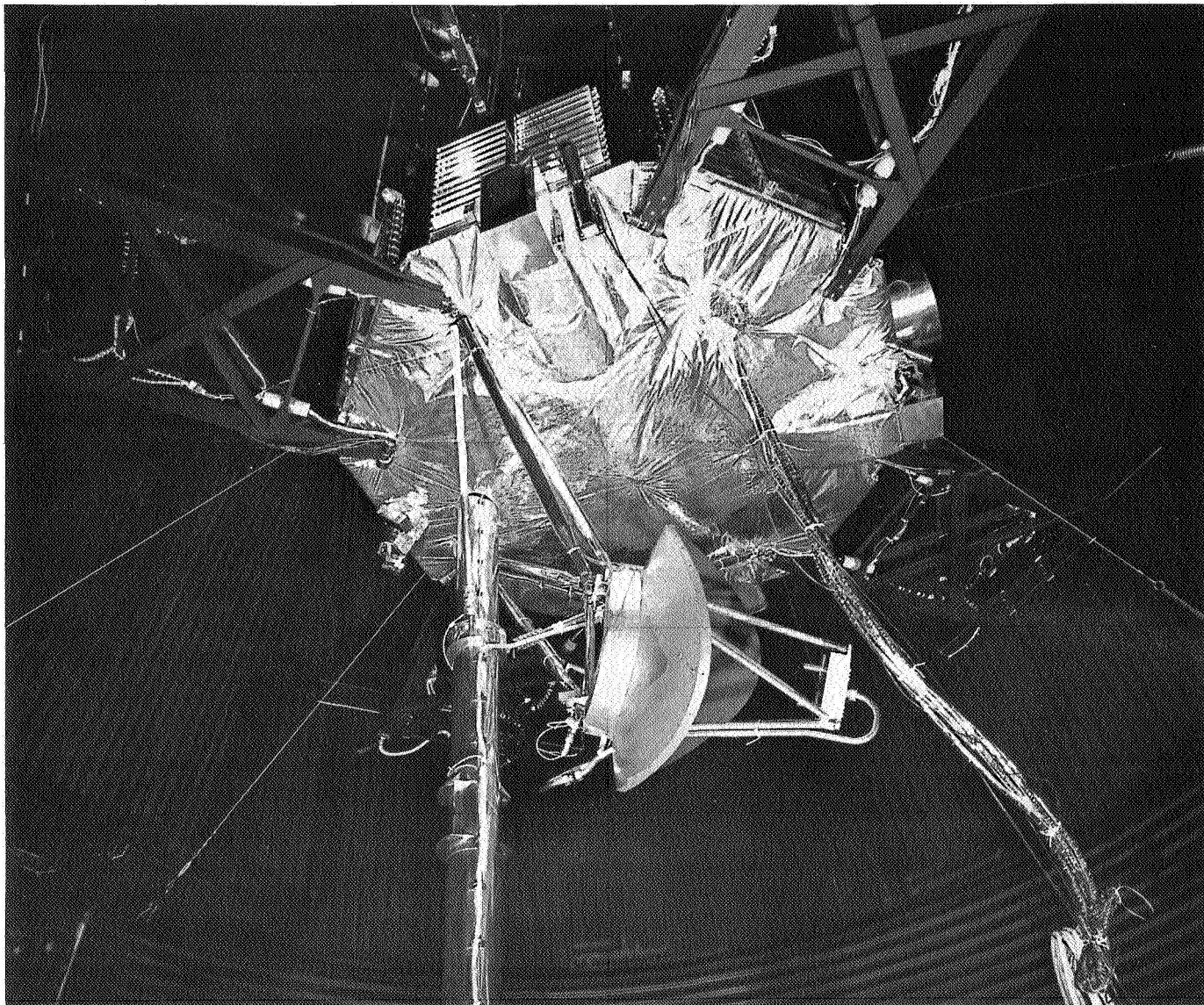
Fig. 13. TCM in JPL 10-ft space simulator
