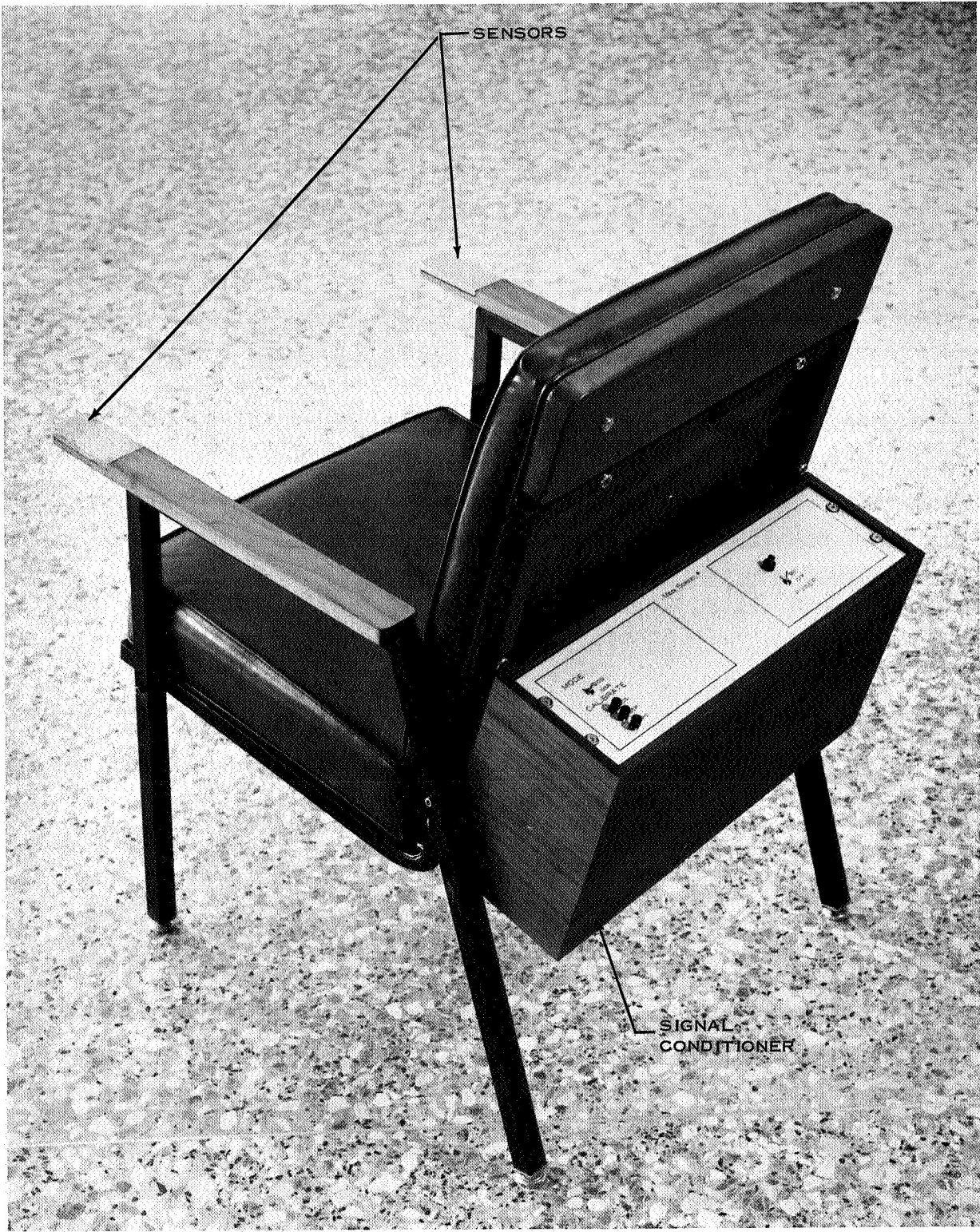
Figure 2-2 Medical Monitoring Chair with Gold Plated Electrodes
