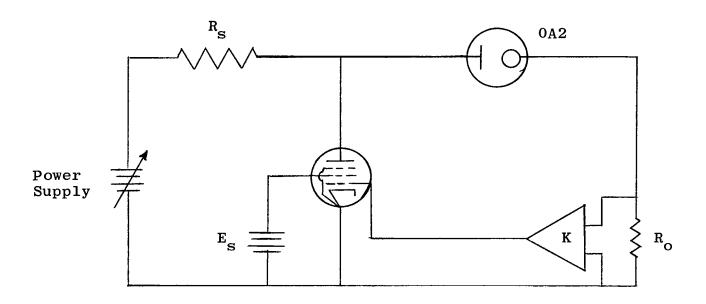
Fig. 1. Schematic Diagram of Feedback System
