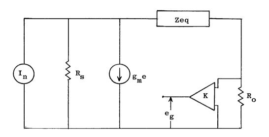
Fig. 4. Small-signal equivalent circuit for "current-current" feedback.
