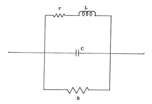
Fig. 3. Small-signal equivalent circuit for an OA2 discharge tube.
