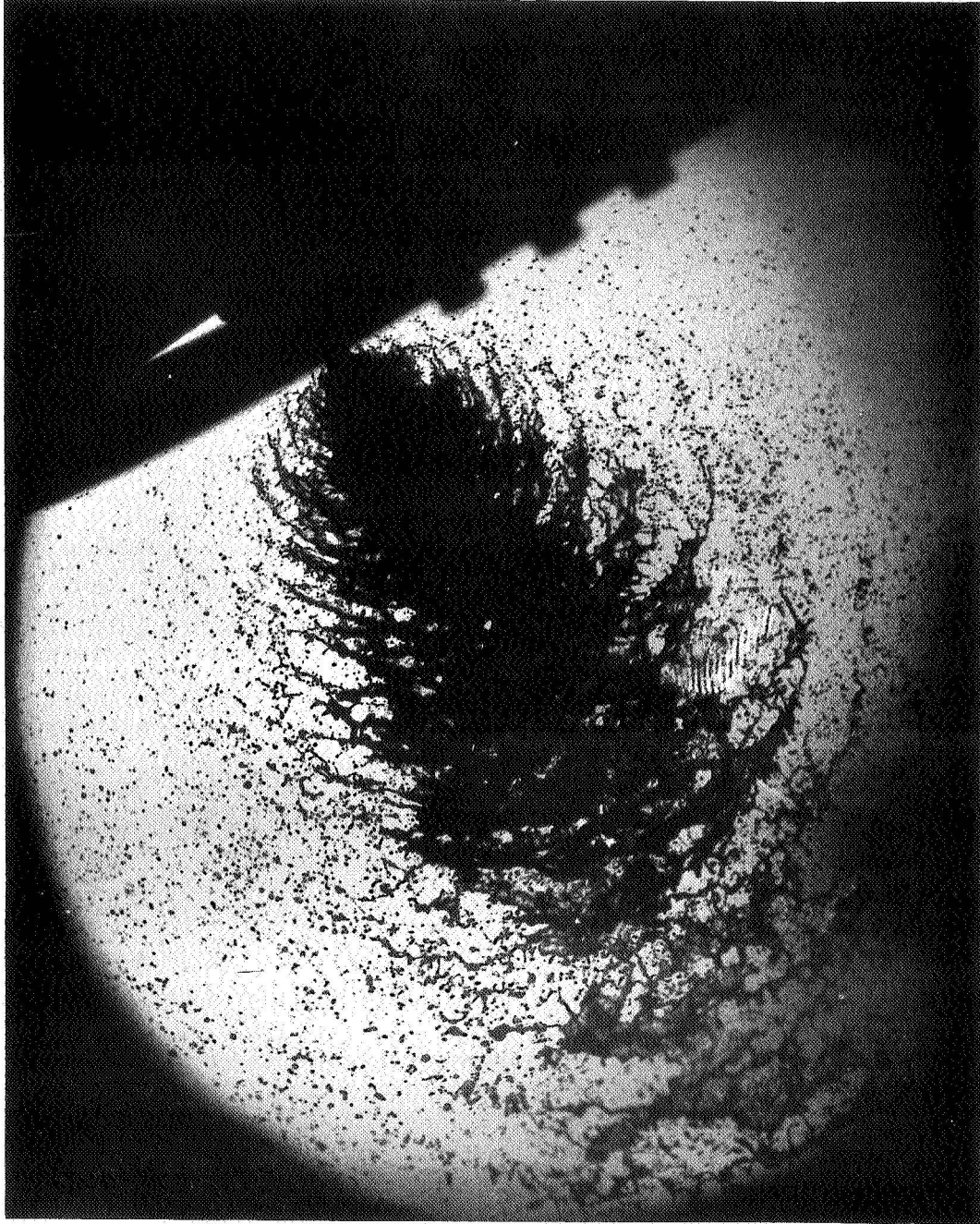
Figure 3-29. Photograph of the reconstruction of hologram B1113I. This photograph illustrates the water flow spray pattern from the single element impinging stream injector operating at a pressure drop of approximately 300 lb/in 2 and a flow rate of 2.35 lb/sec.
