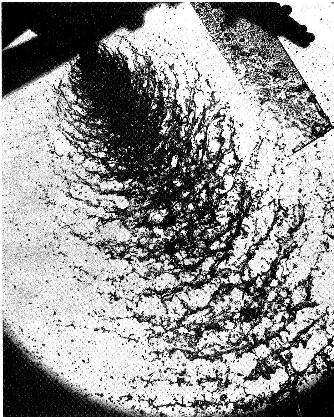
Figure 3-30. Laser-illuminated photograph of the water spray fan produced from a single element doublet during Run B1113L
