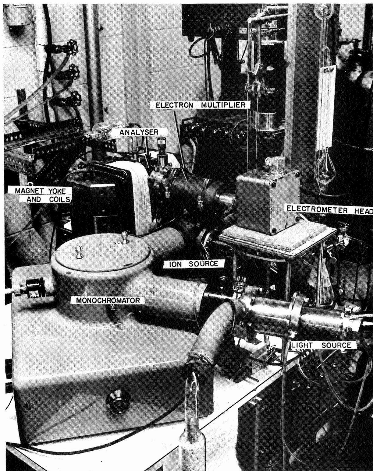
Figure 4. Photograph of photoionization-mass spectrometer setup.
