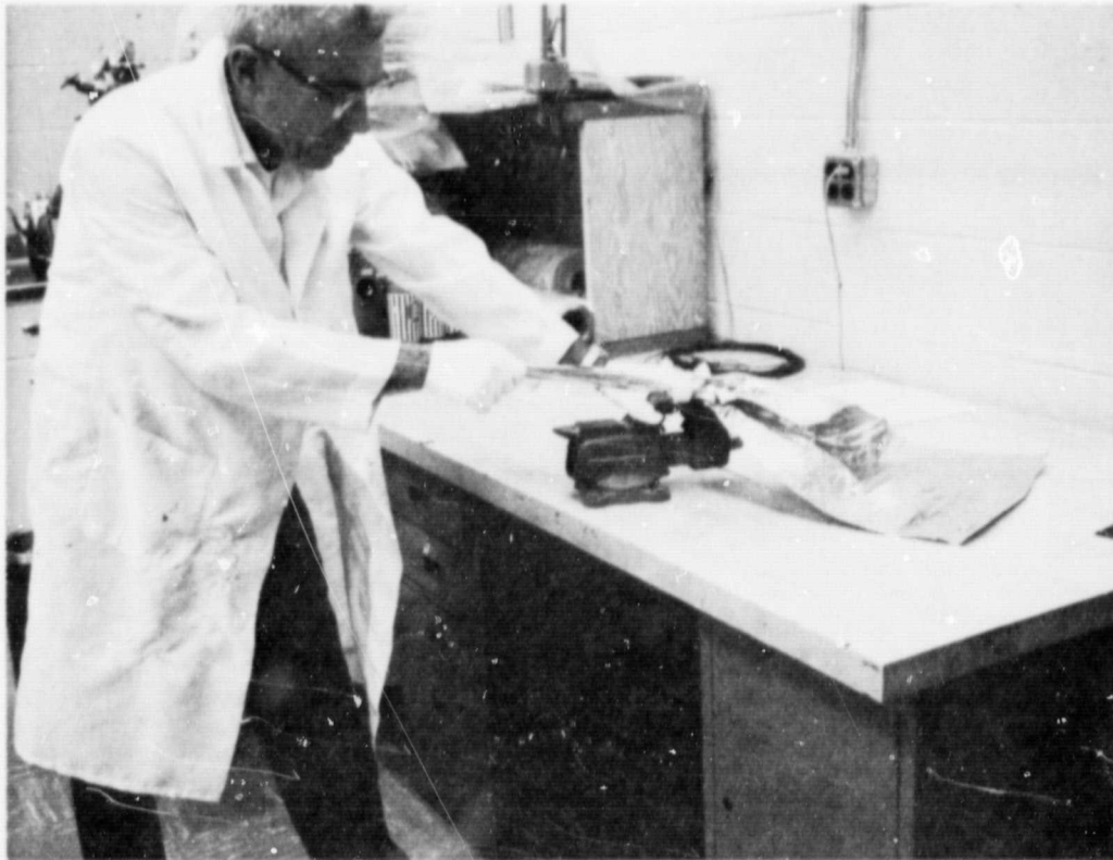
Figure A-4. Crinkling of Insulation by Drawing Through Teflon Die
