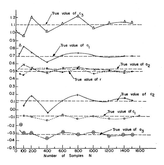
FIGURE 2. GRAPH OF MAXIMUM LIKELIHOOD ESTIMATES OF  $a_1, a_2$ ,  $a_3, c_1, c_2, c_3$ , AND r VS NUMBER OF SAMPLES.
