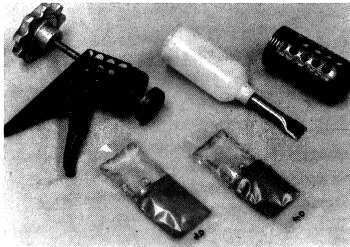
Figure 7. Exploded View of Adhesive Dispenser
