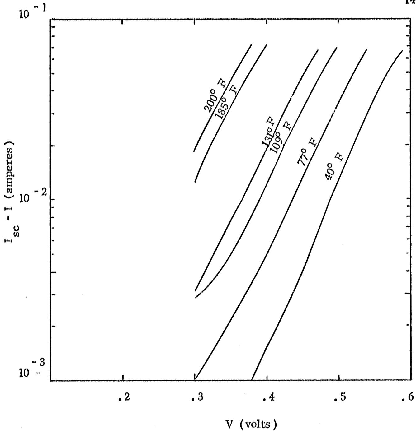
Figure 5. Plots of  $(I_{sc} - I)$  versus voltage  $V$ , from Reynard's laboratory data, using a sun simulator (Ref. 9). Note the slopes of the curves, for various temperatures, are essentially identical near open-circuit.
