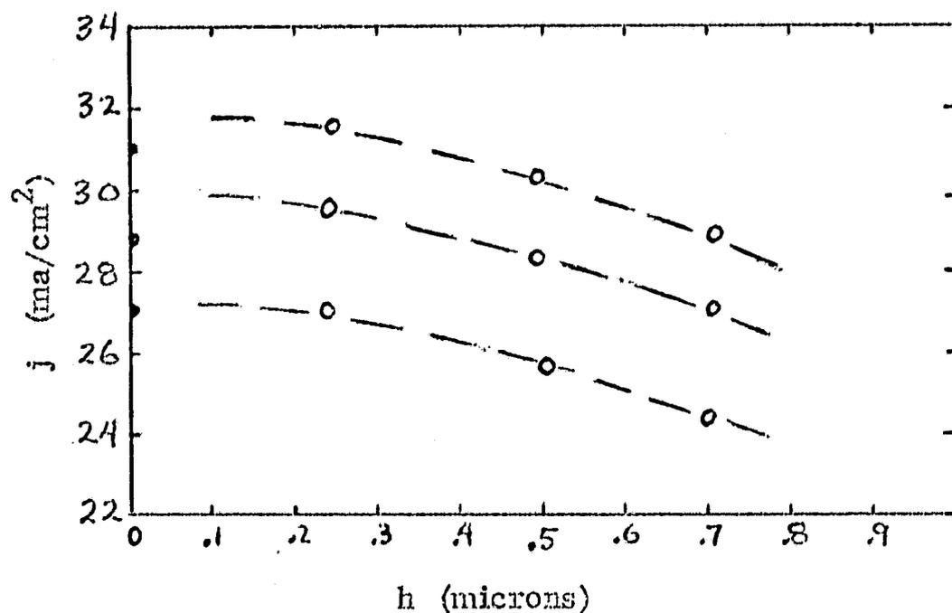
Figure 2. Calculated values of short-circuit current density versus mesh interval  $h$ , for three cells with different base minority carrier diffusion lengths  $L$ .
