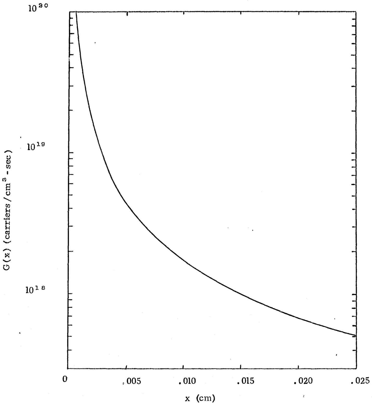
Figure 1. Computed values of the number of minority carriers /  $\text{cm}^3$  - sec produced in silicon by space sunlight as a function of depth  $x$  of penetration. Values from Table 1 were used in equation 11 and reflection was neglected.
