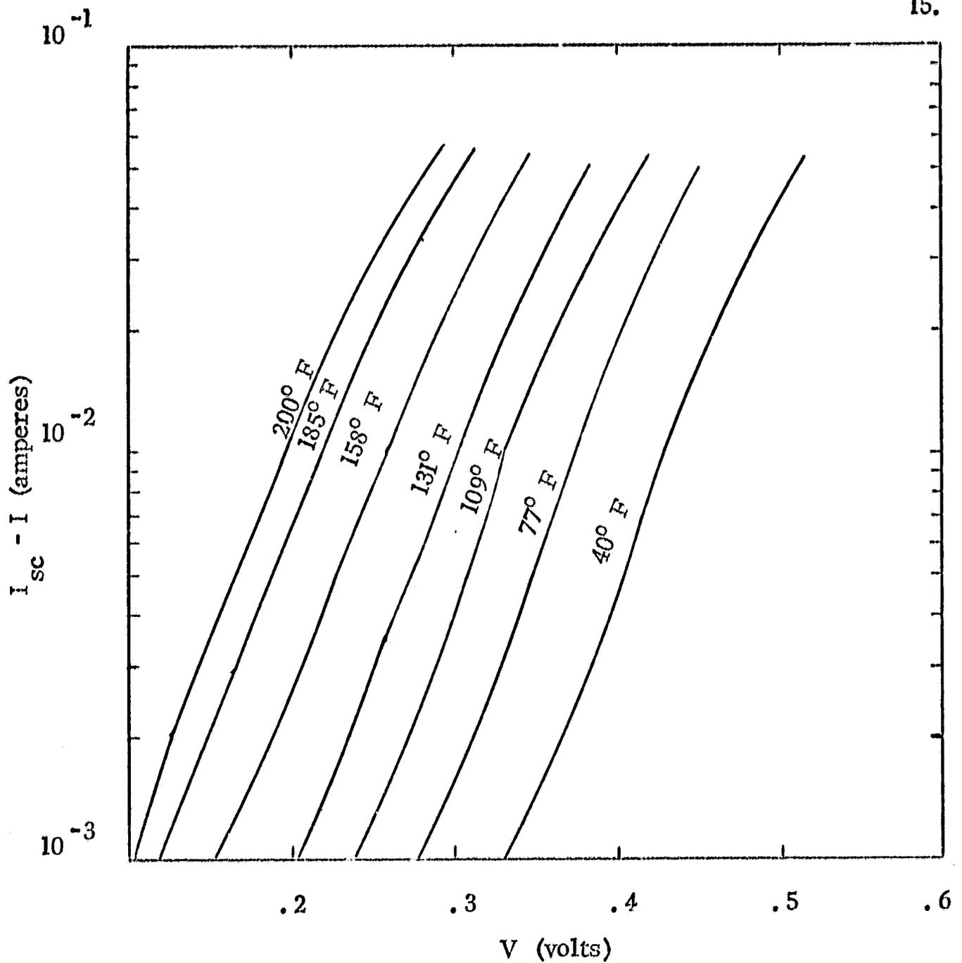
Figure 6. The same presentation as Figure 5, after the cells had been exposed to  $5.2 \times 10^{15}$  electrons/cm<sup>2</sup>. The slopes of the curves near open-circuit voltage again appear independent of temperature and are essentially unchanged from the slopes of Figure 5.
