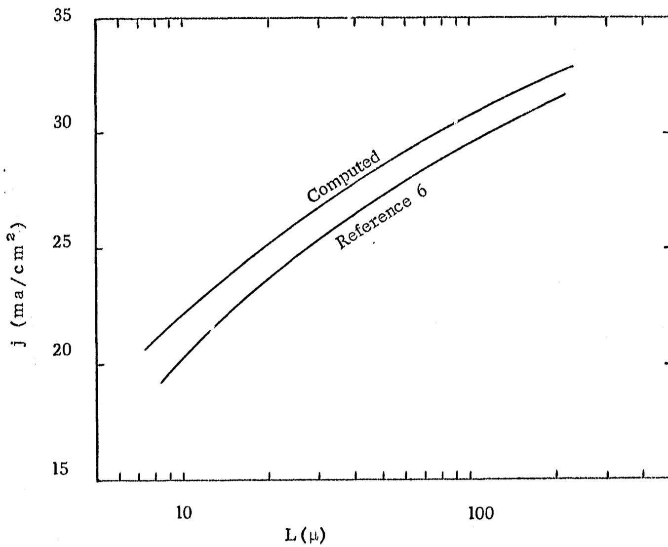
Figure 4. A comparison of computed values of photovoltaic current, versus  $L$ , with reported data from Reference 6. For the computation, the base region of a 10 mil cell was divided into 500 intervals.
