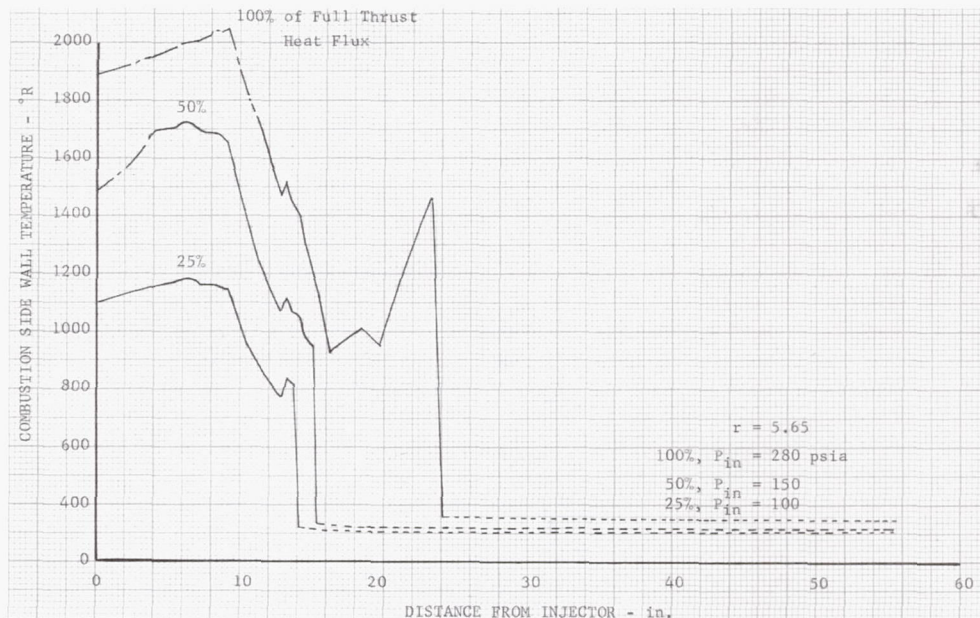
Figure 62. Predicted Start Transient Wall Temperature
