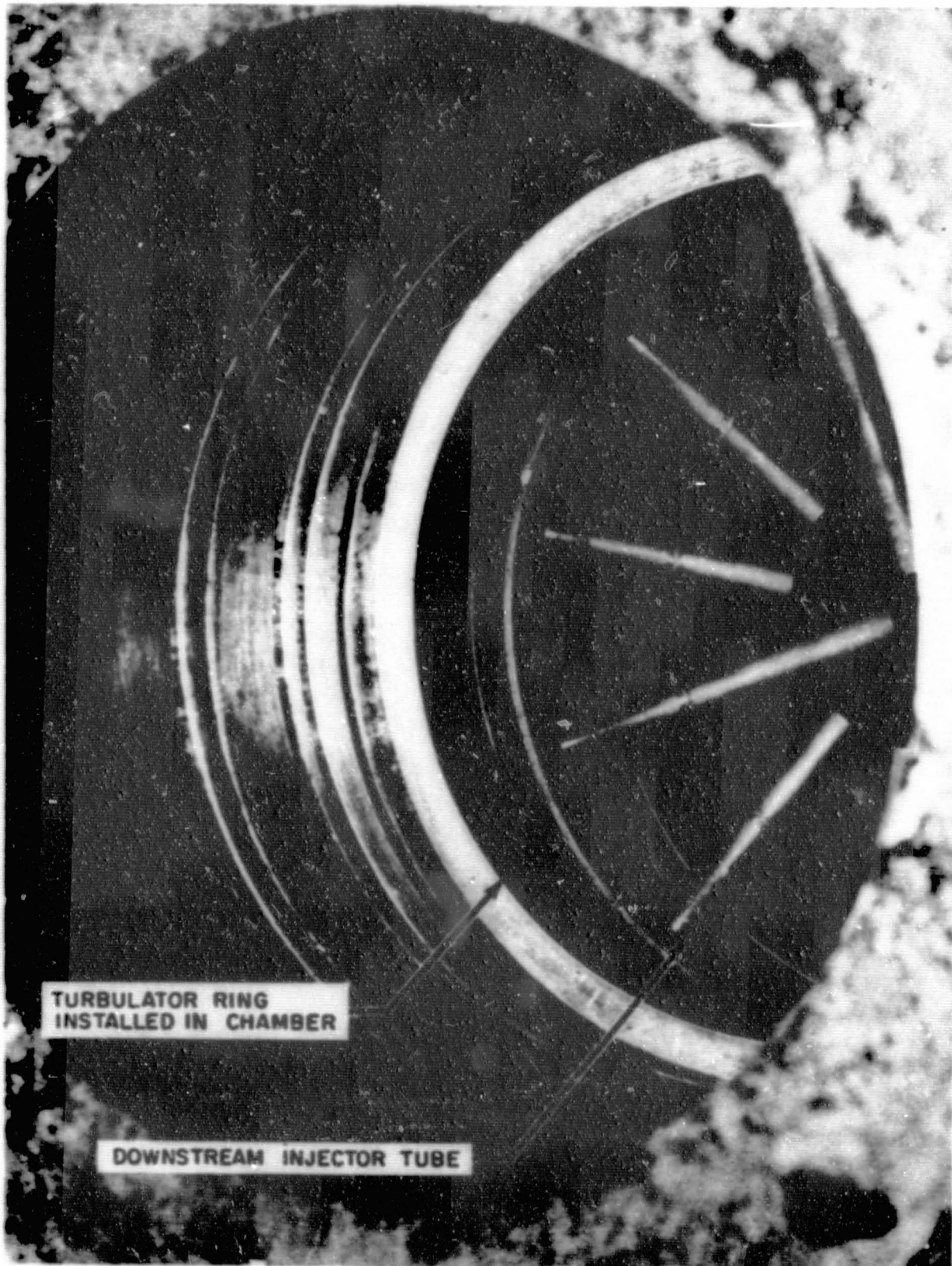
Figure 7. View of Catalyst Bed Chamber (With Catalyst Removed) Showing Installation of a Turbulator Ring
