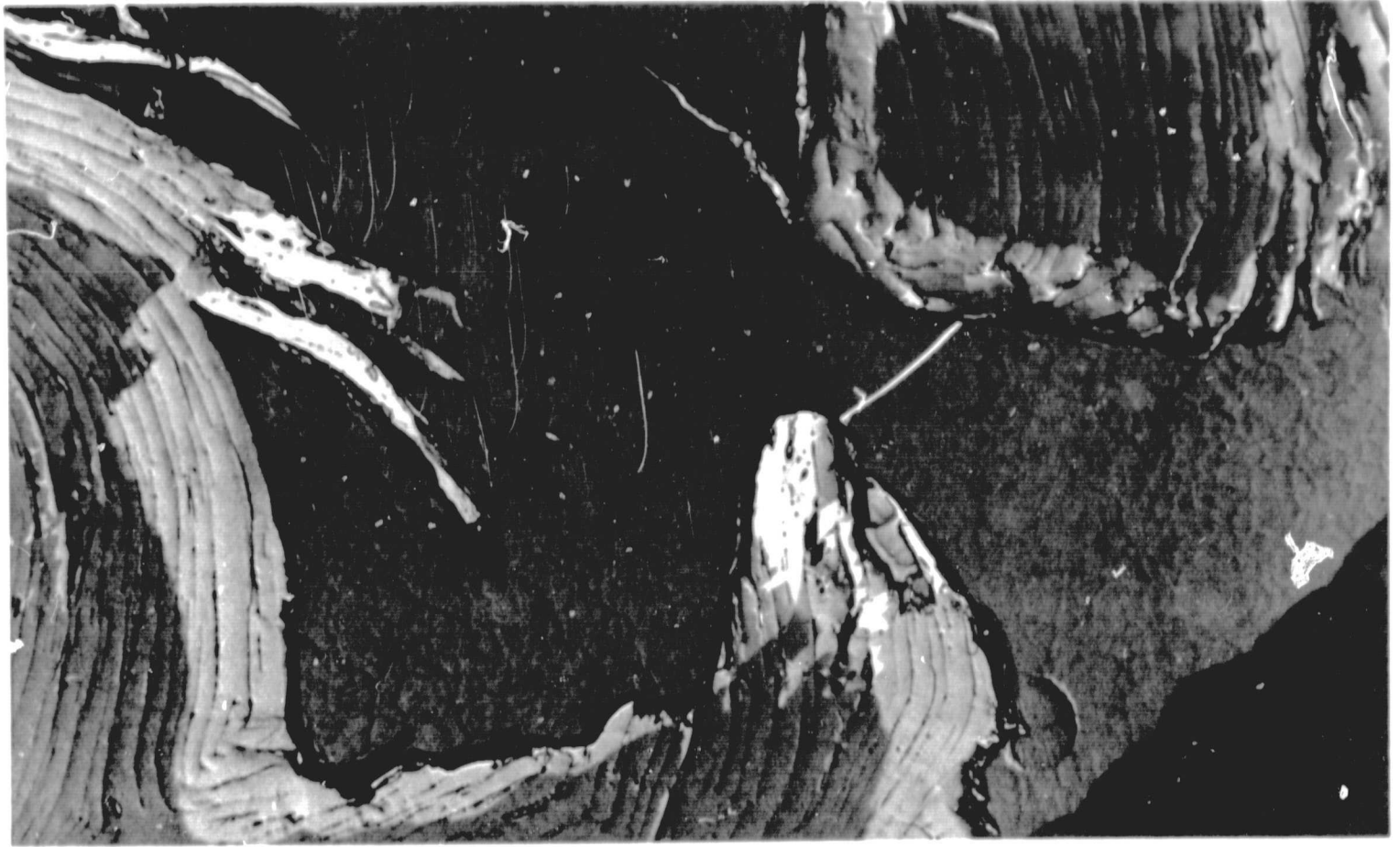
Fig. 14. Cleaved lamellar filler particle. Krypton-ion etch; 7000 X. Reticulated central area is epoxy impregnant separating fracture surfaces. Light areas result from heavy-metal shadowing of replica.
