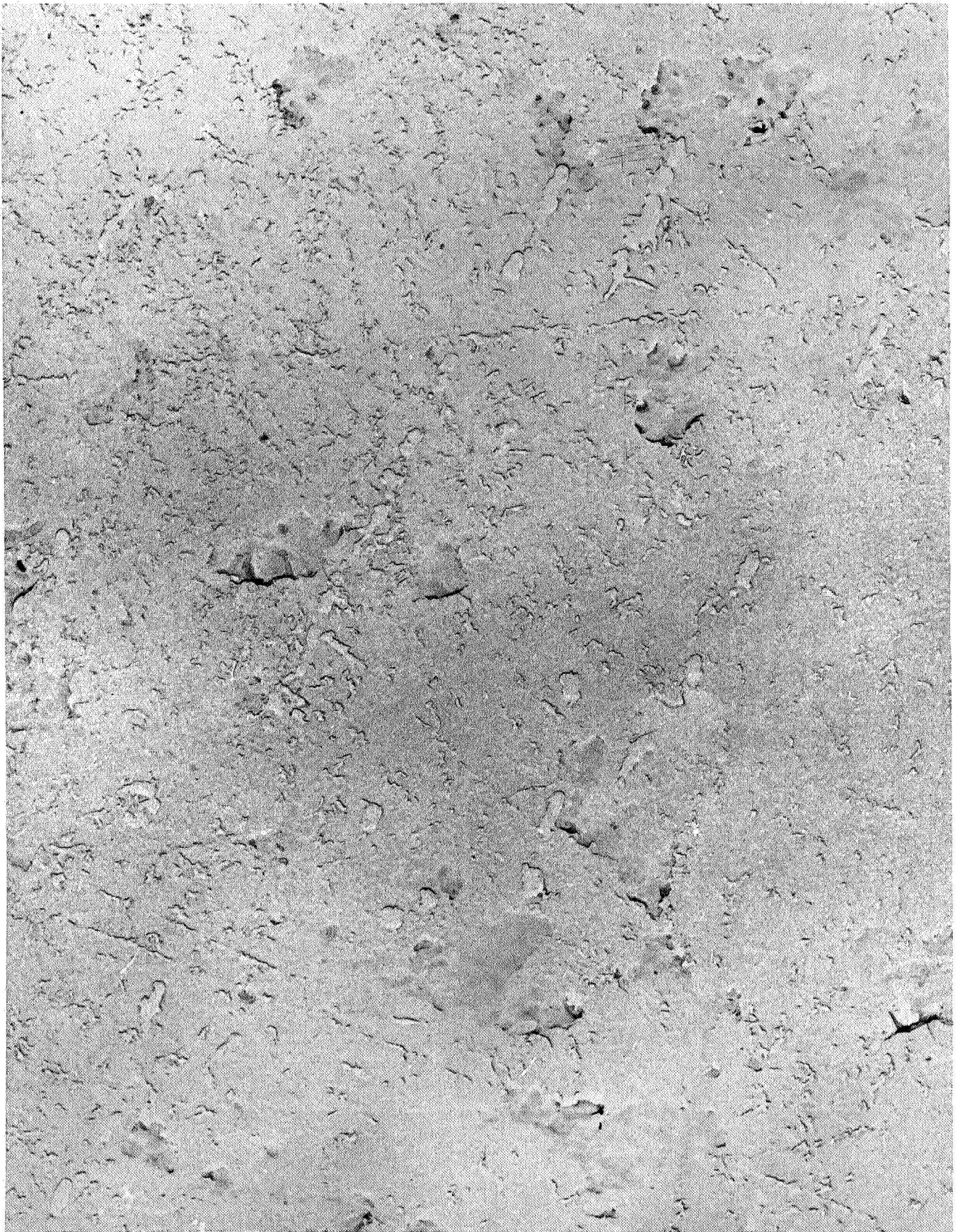
Figure 32. Electron Micrograph of Specimen after 100-hr, 2600 o F Exposure(11,000 mag)
