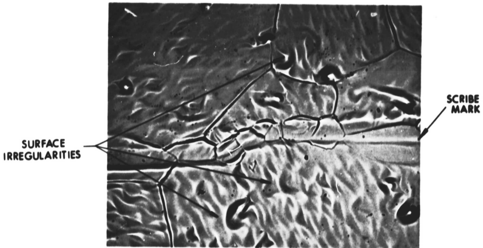
Figure 2. 500X Photomicrograph of Diamond Lapped Vapor-Deposited Rhenium, Sample II, After 2 Hours of Vacuum Outgassing at 2300°C and 60 Hours of Operation at 1900°C
