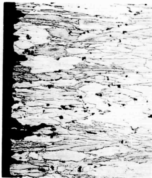
Stressed 75% YS - Exposed 16 days
