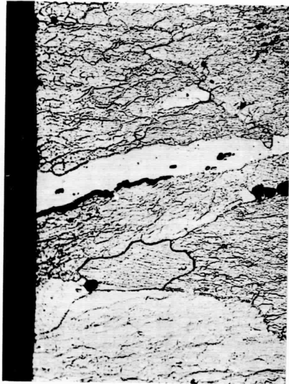
Crack initiation in 7075-T6 stressed to 75% YS S.T. and exposed to LN Na 2 SO 4 solution at nHz ( \gamma 500)
