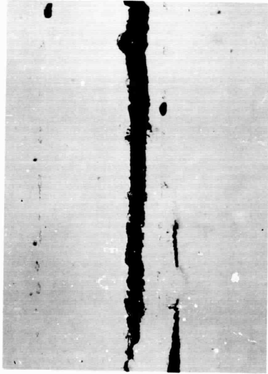
Crack development in 7075-T6 stressed short transversely to 75% YS and exposed in 4N NaCl + 0.5N KNO 3 solution at pH 0.4. (X500)
