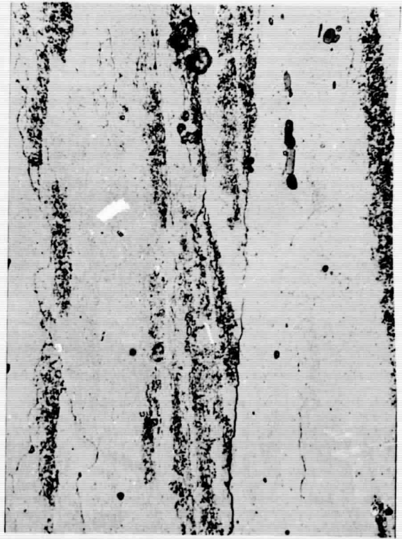
Crack development in 7075-T6 stressed short transversely to 10% YS. (X500)
