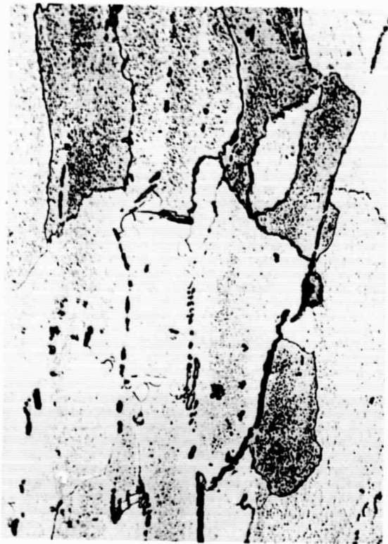
Tuning fork specimen of 2219-T37 stressed short transversely to 75% YS and exposed to 0.5N NaCl + 0.5N Na 2 CrO 4 solution at pH2. (X500)
