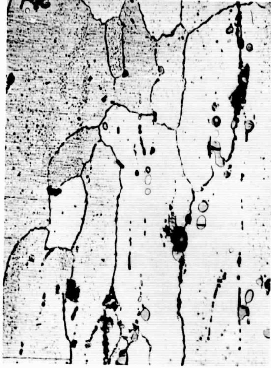
Crack initiation and development in 2219-T37 tuning-fork specimen stressed to 75% YS in short transverse direction and exposed to 4N NaCl + 0.5N KNO_3 solution at pH 0.4. (X500)
