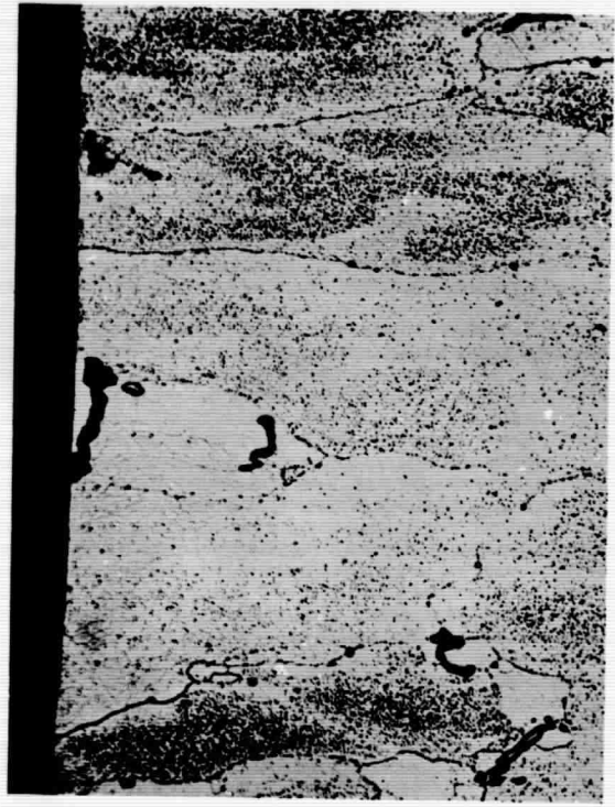
Development of pitting attack in 7039-T6 plate exposed unstressed to pH2 solution of 0.5N NaCl + 0.5N Na2CrO4 (X500).
