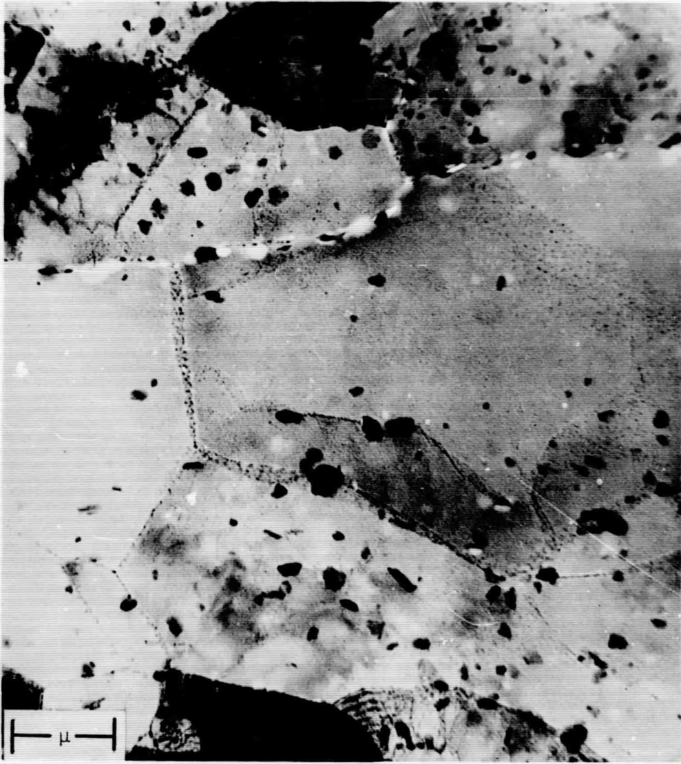
Electron transmission microstructure of 7039-T6 plate showing polygonized structure, dispersoid distribution and occasional dislocations.
