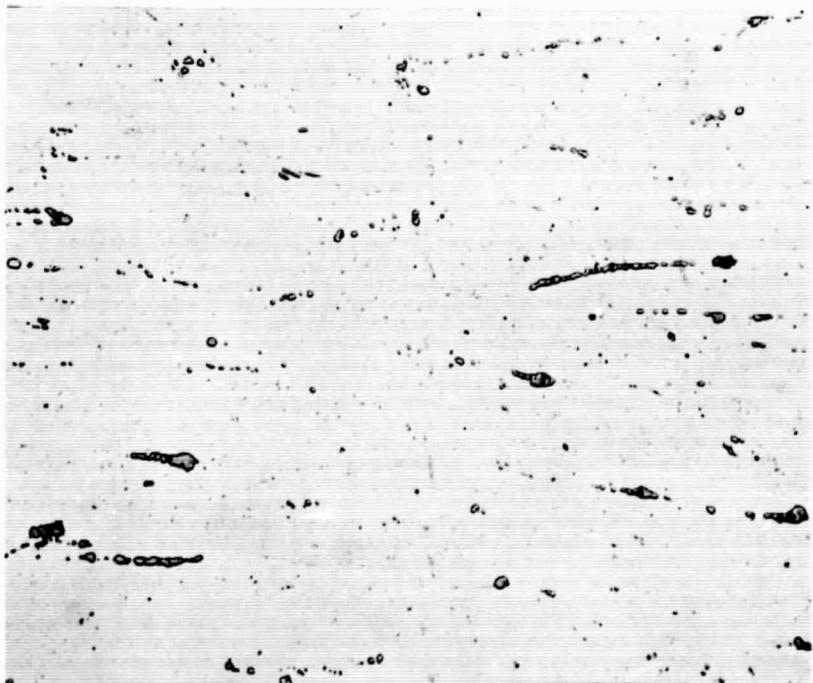
Unstressed corrosion in 1N \text{Na}_2\text{SO}_4 solution at pH2. (X500)
