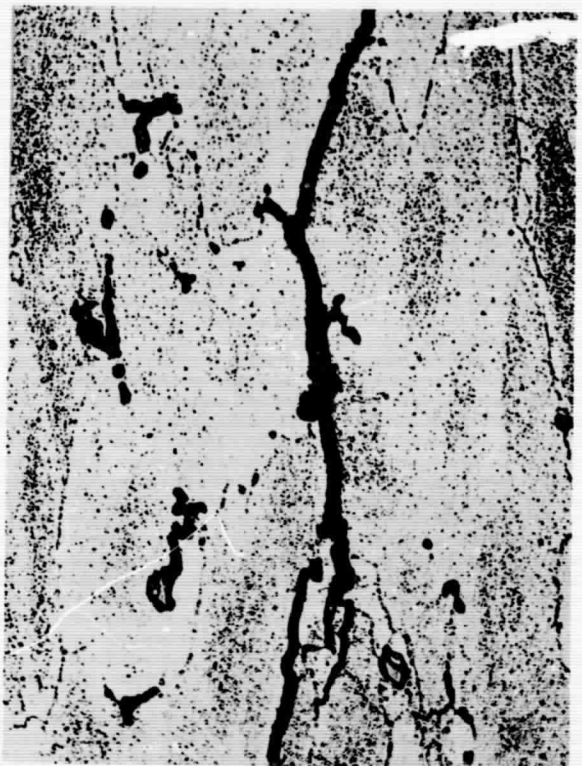
Crack initiation in 7039-T6 plate stressed short transversely to 75% YS and exposed to pH2 solution containing 0.5N NaCl + 0.5N Na 2 CrO 4 (X500).
