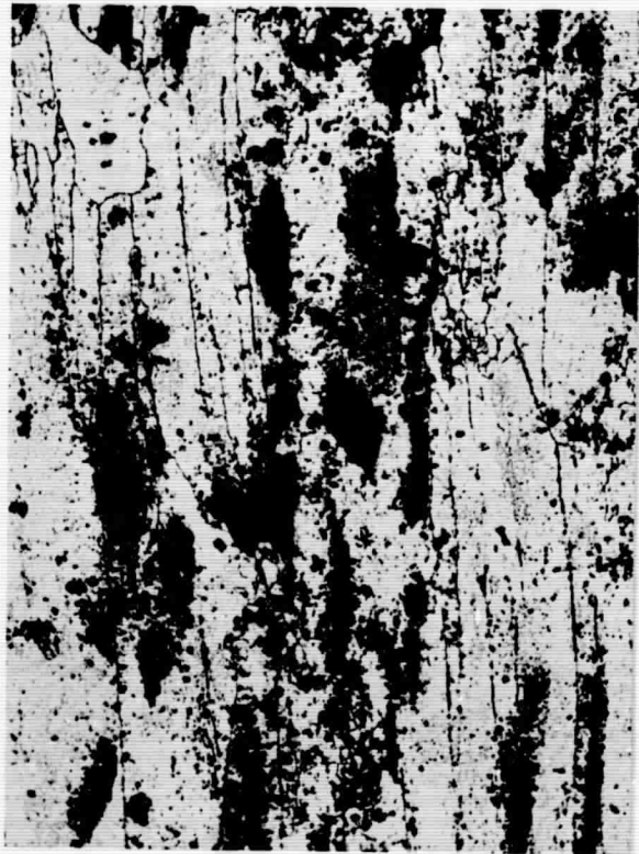
Development of intergranular, interfragmentary and matrix pitting attack of 7079-T6 plate exposed unstressed to pH 1 NaCl-AlCl 3 solution (X500).
