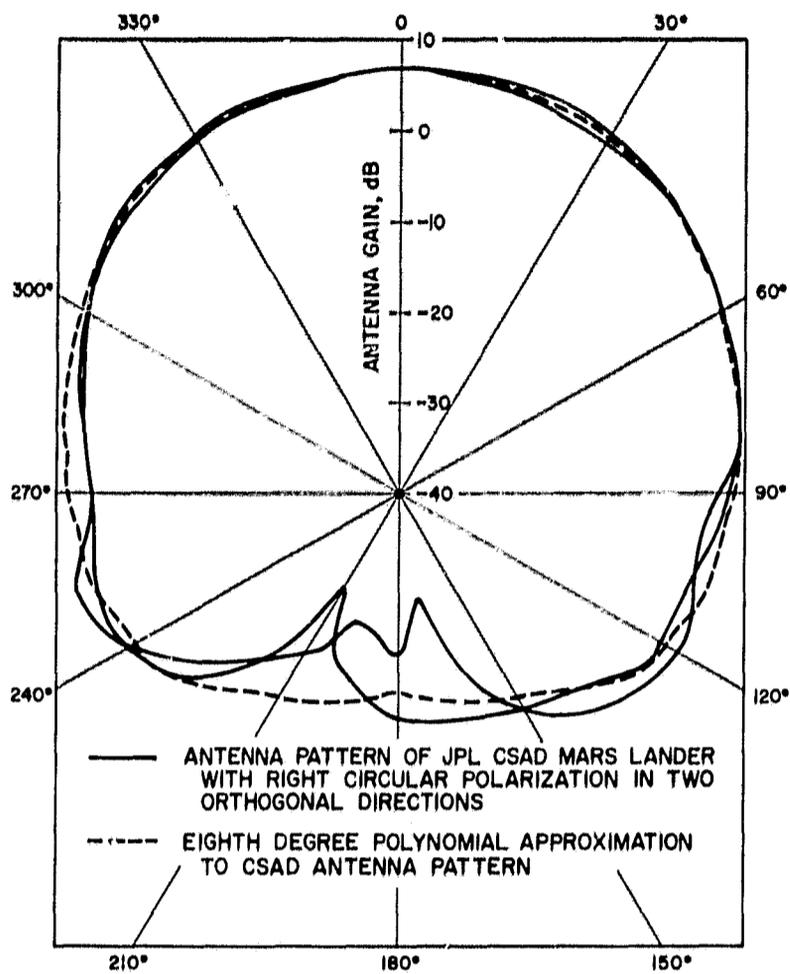
**Fig. B-2. Antenna gain characteristics**
