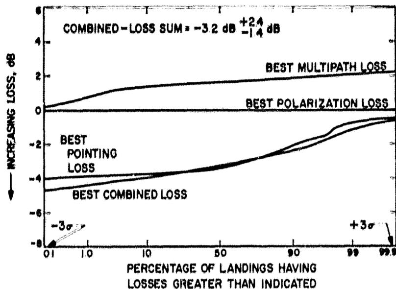
Fig. 8. Pointing, multipath, polarization, and combined loss distributions for circular polarization 21.3 h after landing
