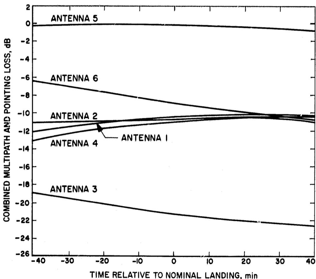
Fig. C-1. Multipath and pointing losses vs planet rotation
