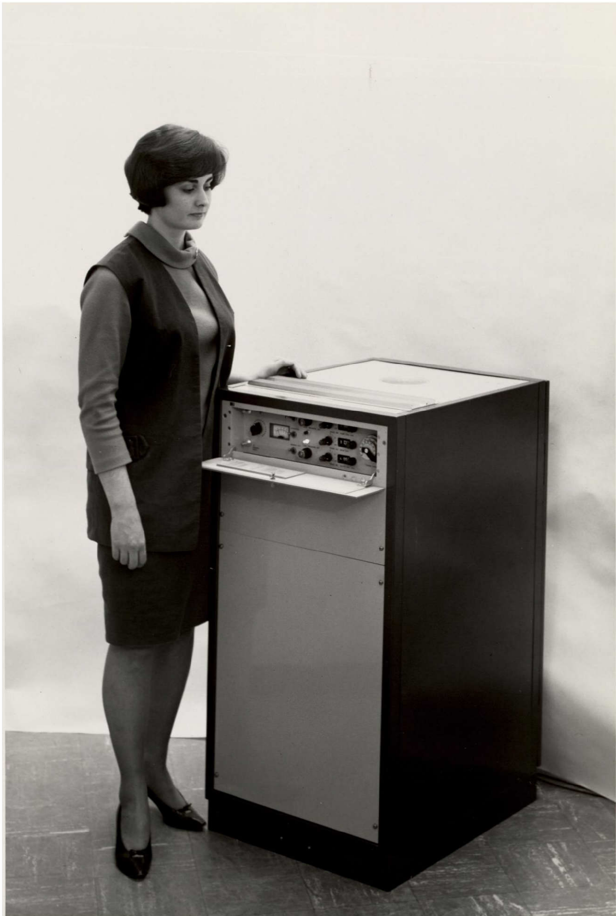
Fig. 1. Completed Atomic Hydrogen Maser for Field Use.
