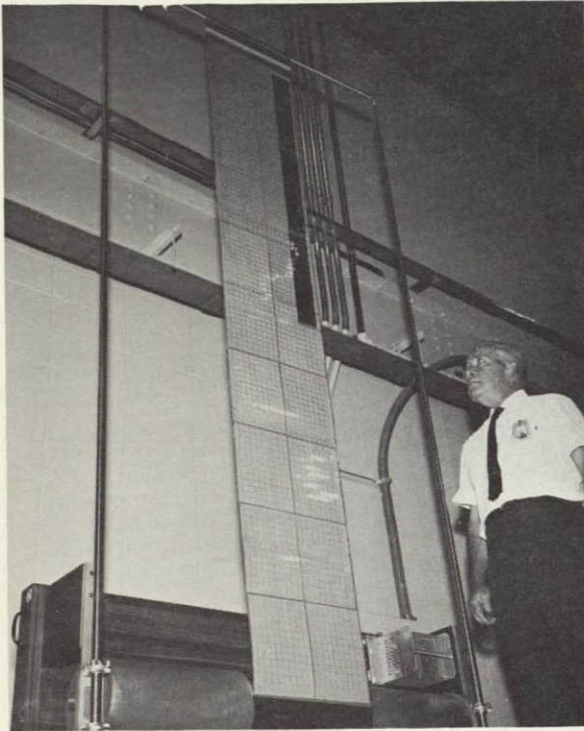
Figure 4.7-10. Engineering Model of Rollup Solar Array
