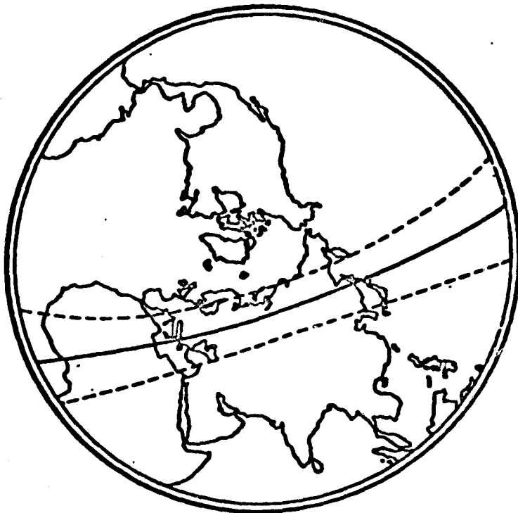
Fig. 1. Region scanned during the motion of a meteorological satellite over the northern hemisphere in a circular orbit and altitude of 600 km.
