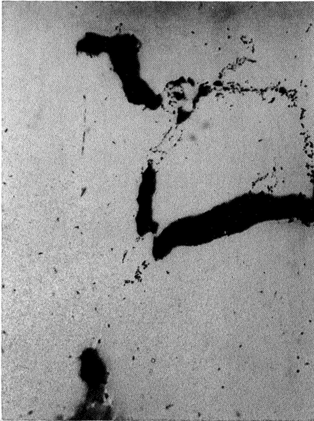
Saturn S IV B Helium S/N 2 Storage Vessel Section of green protrusion on fracture face
