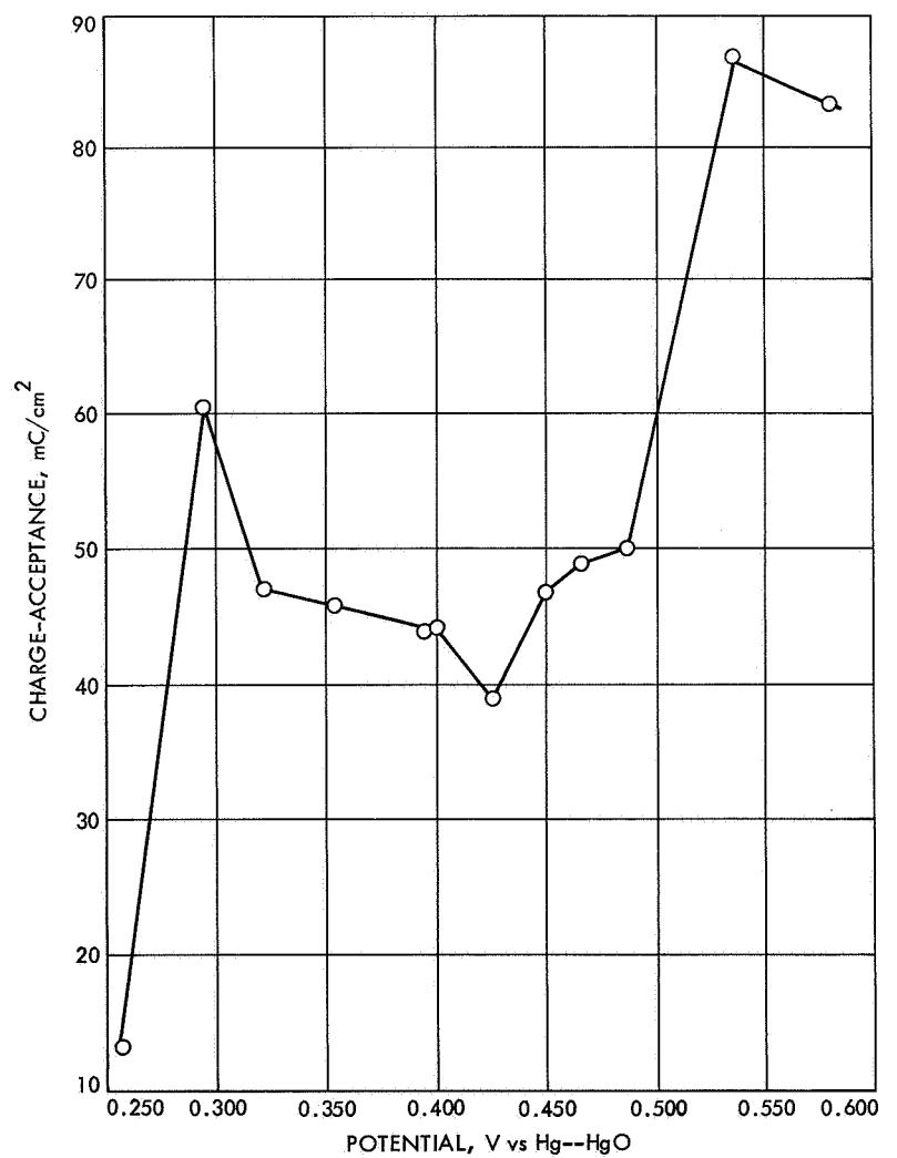
Fig. 19. Plot of charge-acceptance per unit area of smooth electrodes vs applied potential
