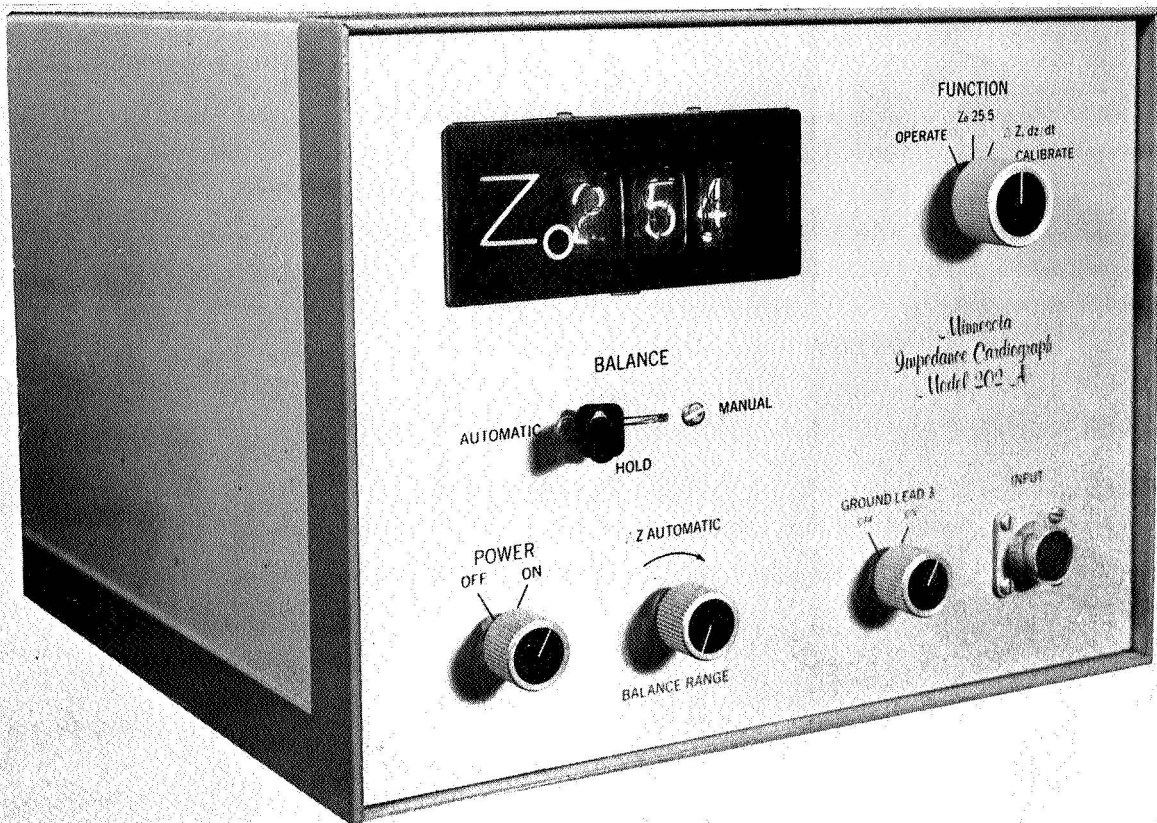
Fig. 4 The front panel of the Impedance Cardiograph showing the controls and the automatic digital display of Z_0 .
