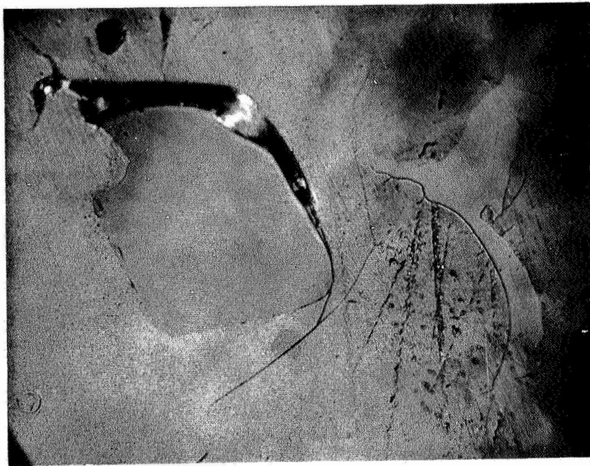
Fig. 1 (\text{CoSi}_2)_{.1}(\text{2Ge})_{.9} as cast, polarized light. 700 X
