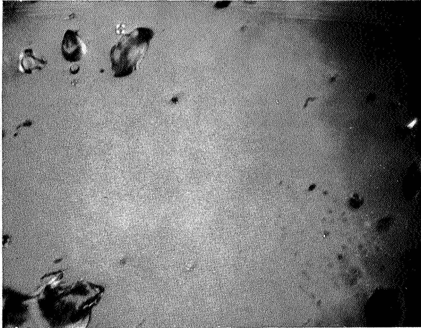
Fig. 8 (\text{CoSi})_{.5}(\text{CoGe})_{.5} 864 hours, 900°C, polarized light. Note .5 single .5 phase appearance. 700 X
