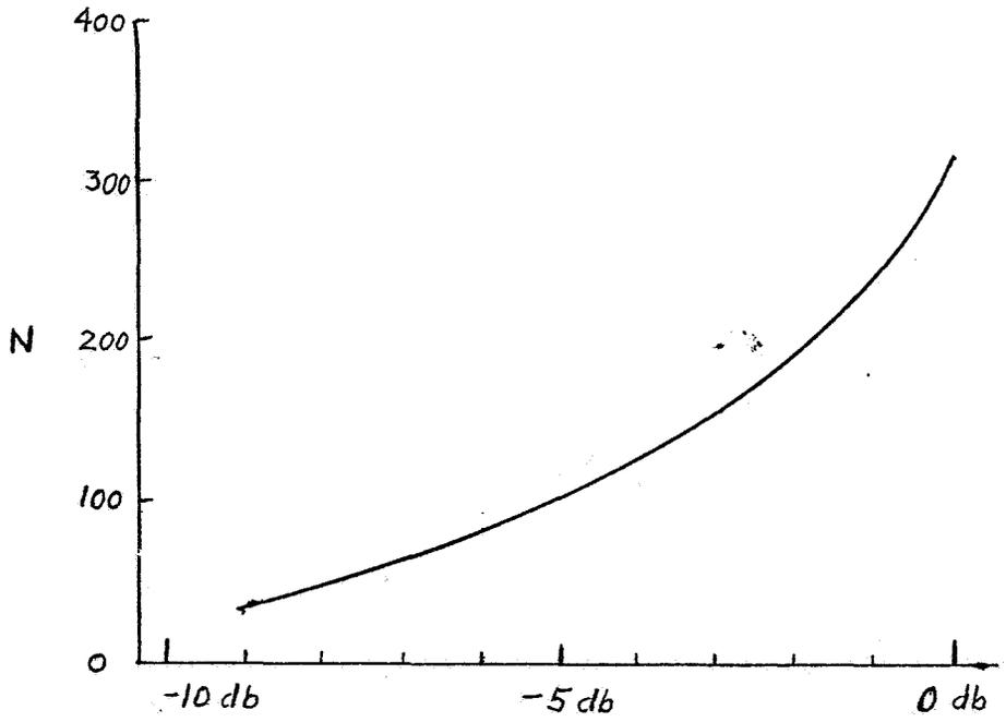
Ratio of Reflection from Conductors to Reflection from no Conductors
