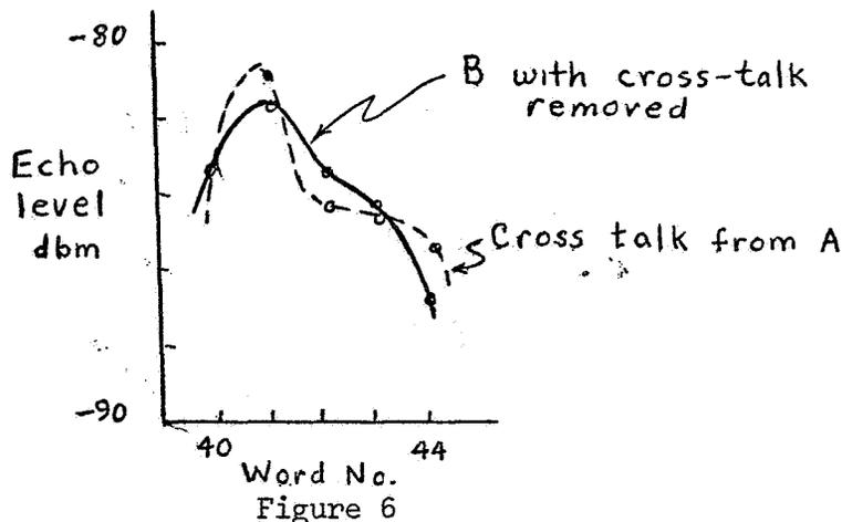
The principal conclusion to be drawn from the waveforms sketched in Figure 6 is that the independent component of B appears to be specular, i.e., a replica of the transmitted pulse, rather than scattered return. The characteristic for the initial build-up in the case of scattered
