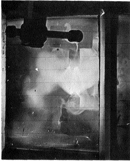
P_{\infty} = 1.0 \text{ atm}, I = 300 \text{ A}, \text{ gap} = 1.2''
