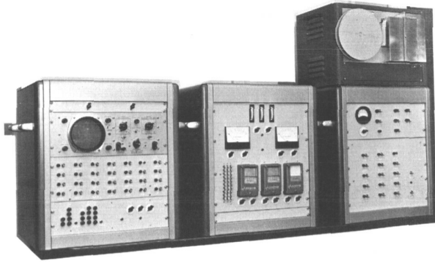
Fig. 5 A Polariscope Ground Station. The oscilloscope serves as a television screen, below which are the toggle switches for the command system, and under that is a binary clock-timer. The middle panel has quick-look indicators and recorders, and the panel on the right has special command switches operated by a separate observer. At the top, a papertape punch is shown; a magnetic tape recorder is also used.
