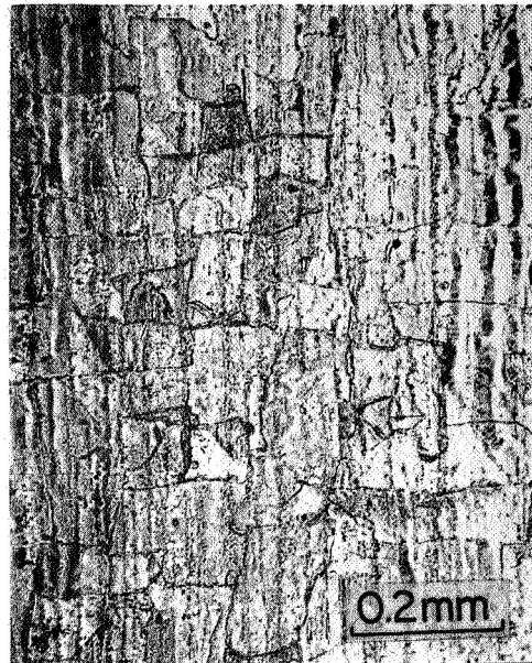
(b) After Reversed Creep, T=0.5T_m, \tau_a = \pm 640 \text{ psi}, \Delta\gamma=0.047
