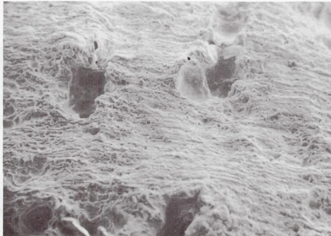
LIQUID IMPACT EROSION OF 1100-0 ALUMINUM IMPINGEMENT VELOCITY 450 fps FOR 3 MINUTES ( MAGNIFICATION: 88X )
