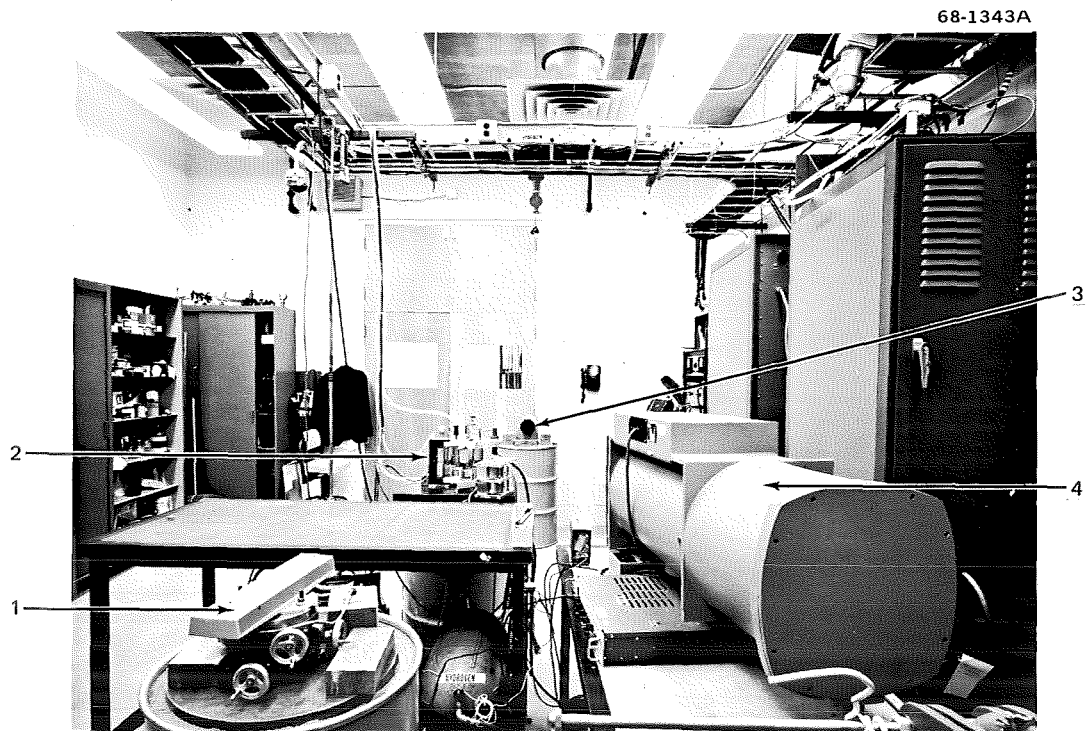
Figure A3. Equipment for Measuring Time-Dependent Optical Transmittance
