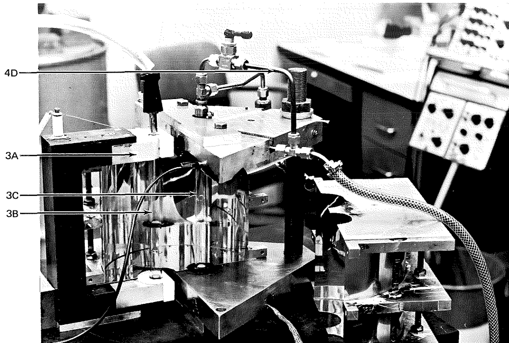
Figure A2. Elliptical Reflector, Flash Lamp, and Test Cell
