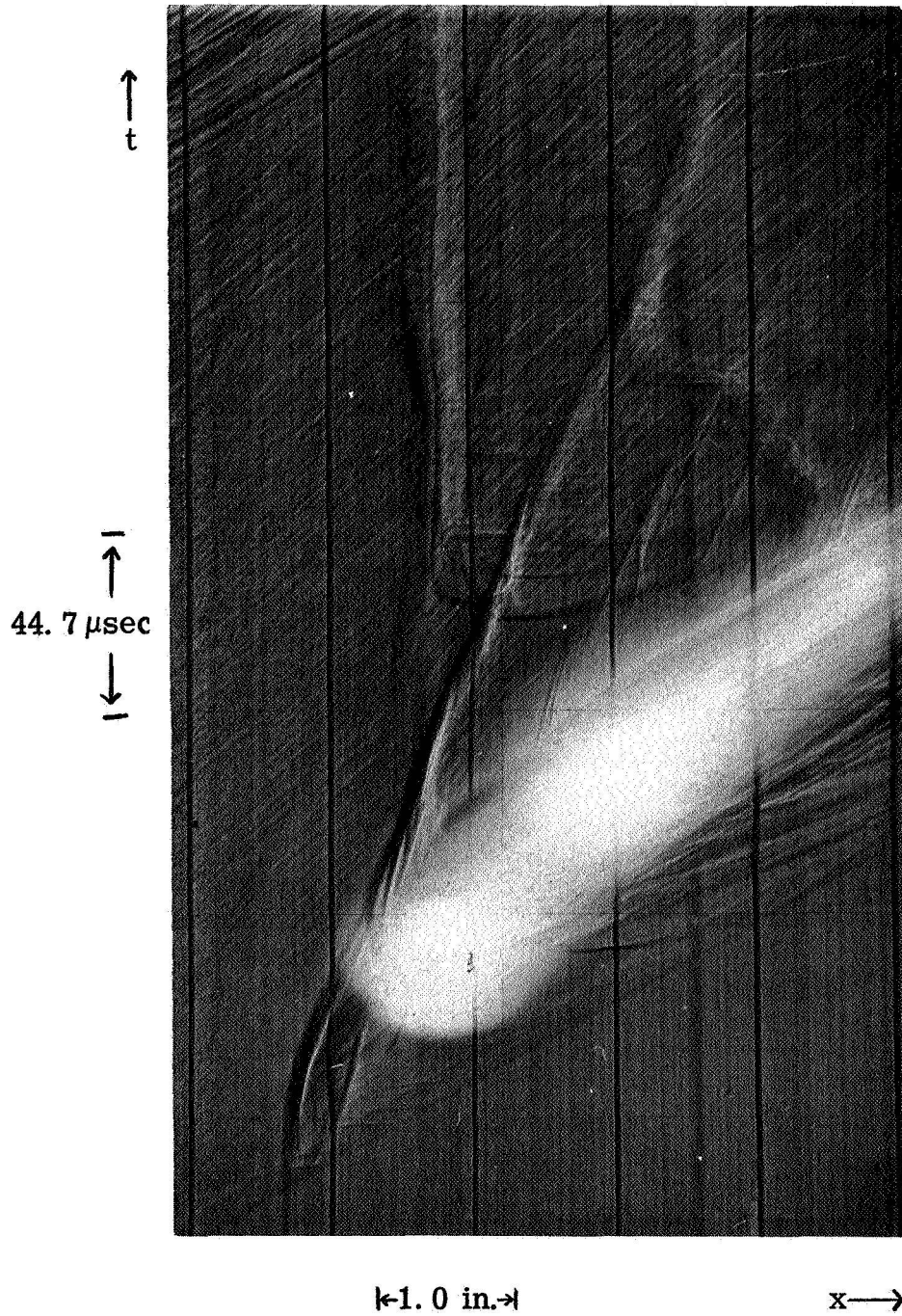
Figure 3. Shock Passing over a DECH Drop in O_2 . Run No. 143, d = 1580 \mu , M_1 = 4.05 , p_1 = 20 in. O_2 , w_1 = 4370 ft/sec, M_2 = 1.562 , w_2 = 3390 ft/sec
