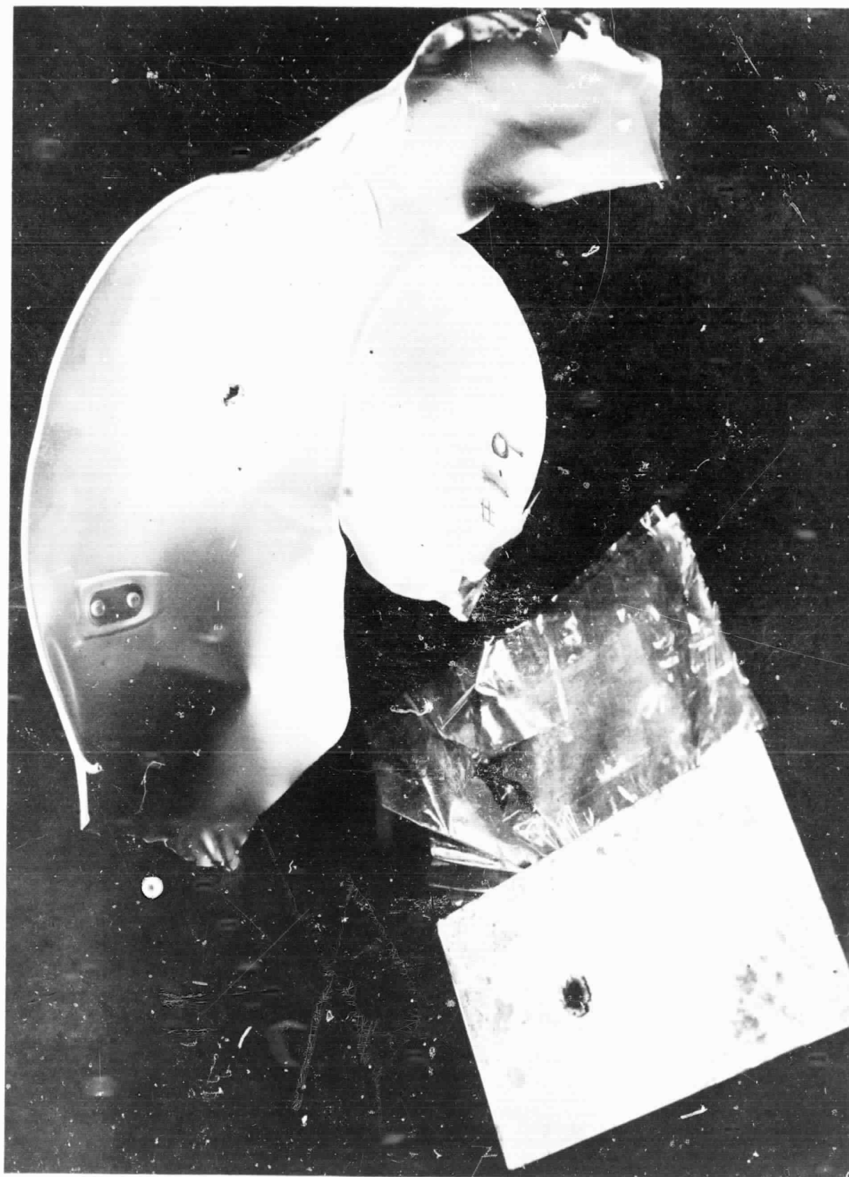
FIGURE 8 SPECIMEN 19 AFTER LOX BALLISTIC IMPACT TEST
