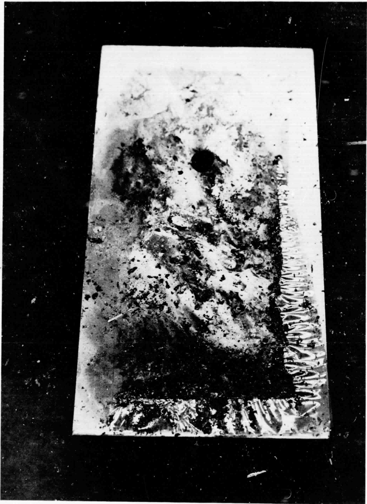
FIGURE 7. SPECIMEN 18 AFTER LOX BALLISTIC IMPACT TESTING
