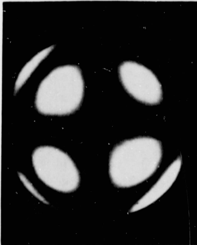
FIG. 6 Conoscopic image obtained by viewing LiTaO 3 in convergent polarized light. (1 mm thick sample viewed parallel to the c axis.)
