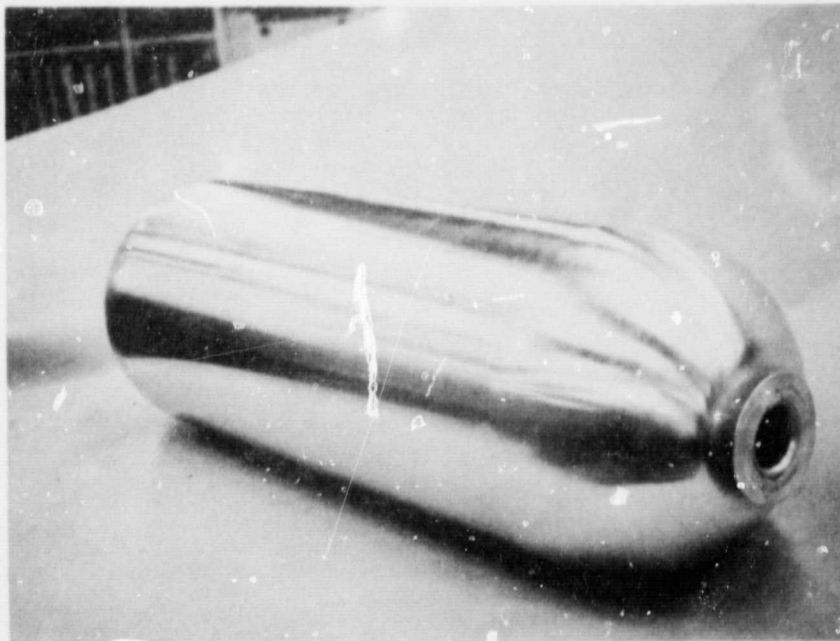
Figure 2 RCS Size Mandrel, Polished for Plating (P/N SE-1032)
