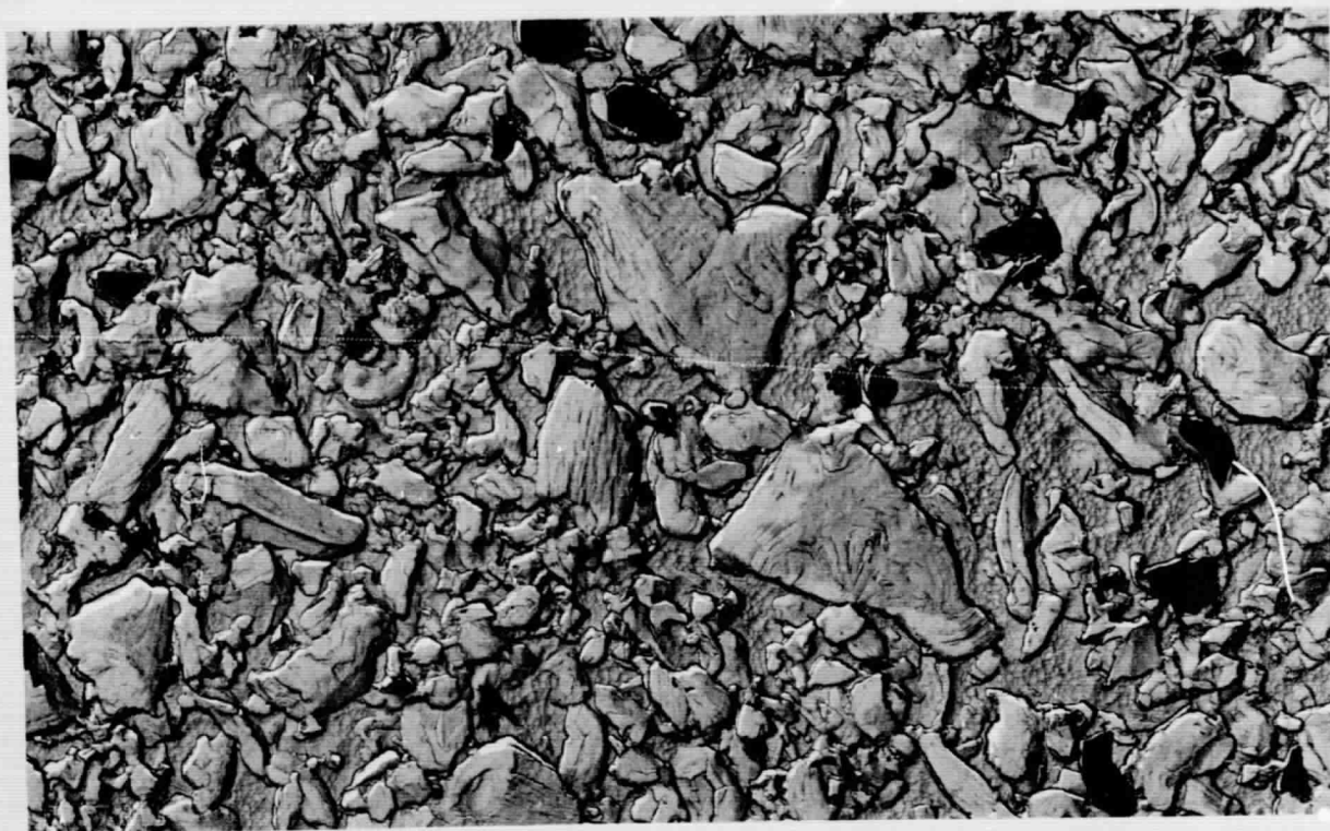
Fig. 3. Typical particle shapes of ground Santa Maria coke. Rough gray areas between particles are epoxy mounting resin. Xenon-ion etch, 3200X.
