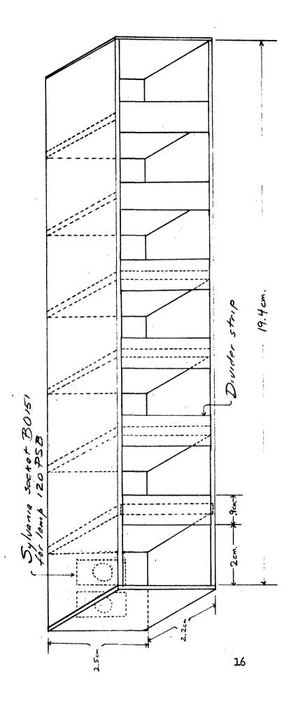
Fig. 5 Details of high the compartment
