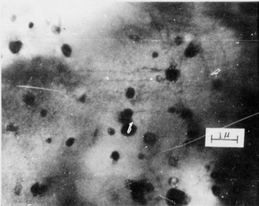
FIGURE 17. STRUCTURES FREQUENTLY OBSERVED IN D43 PRIOR TO CREEP TESTING SHOWING REGIONS WITH AND WITHOUT SUBGRAINS
