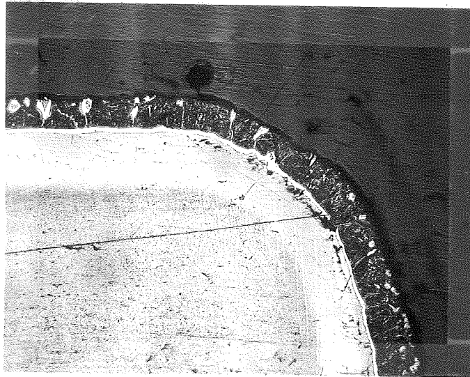
After Diffusion Treatment Note tunnel at edge.
