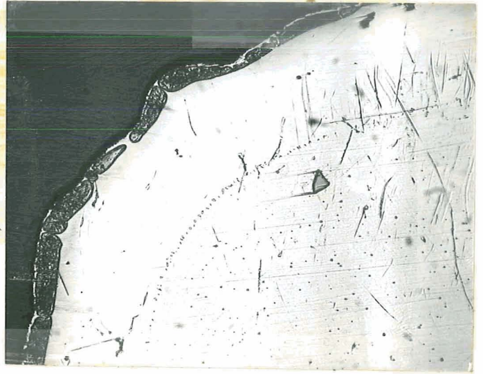
TD-Ni - Ni-30Cr-1Si First Step Coating Sample #101
