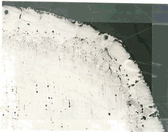
TD-NiCr - Ni-20Cr-3Si First Step Coating Sample #111
