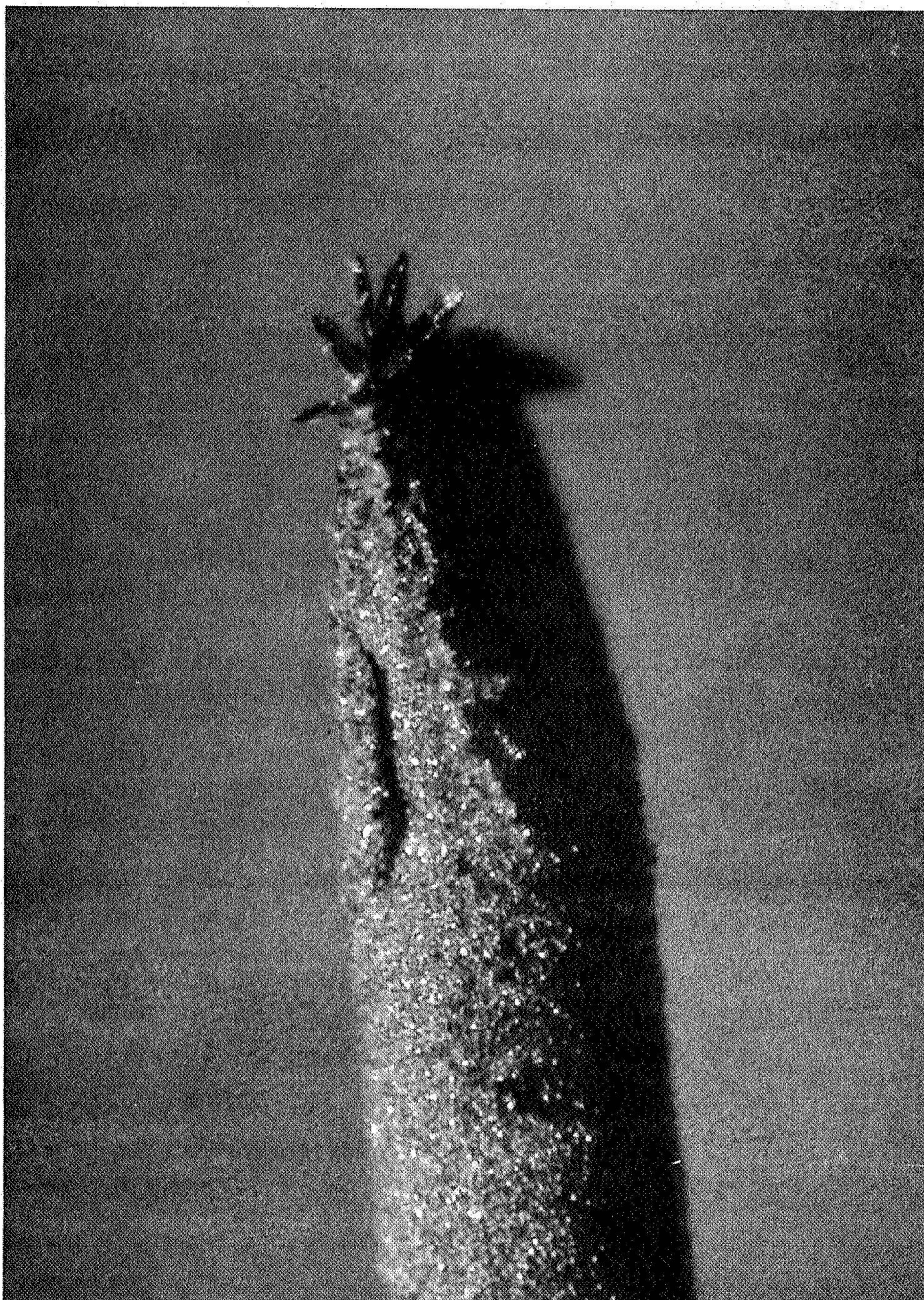
Figure 2. Photograph of the Whiskers Deposited on End of Pt Cathode in Cell E8 From \text{AgNO}_3/\text{NH}_3 Solution at 140^\circ\text{C} .
