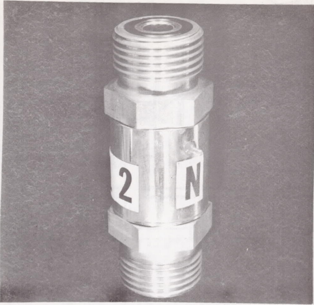
Figure 18. A Photograph of a Complete Transducer and Housing
