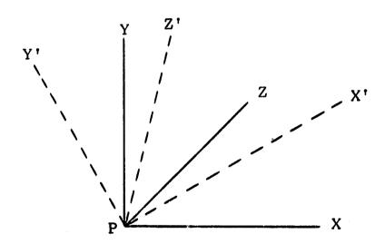
Simultaneous Translation and Rotation. If the origin of the X', Y', Z' system is not that of the X,Y,Z system but has the coordinates  $X = X_0$ ,  $Y = Y_0$ ,  $Z = Z_0$  in the X,Y,Z system, the transformation equations become:
