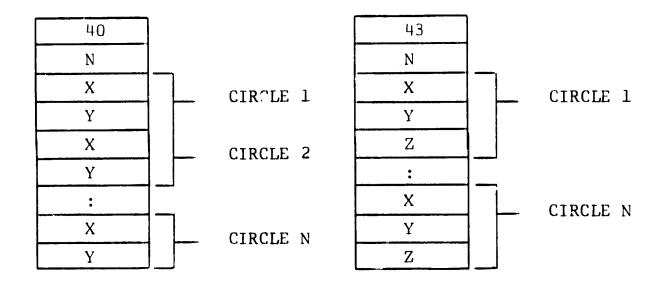
The range of X and Y after translation is 0 to 1023 and the range of RADIUS is 0 to 511. If a value is outside its range, the out-of-range edges are forced to the nearest edge (0 to 1023).
