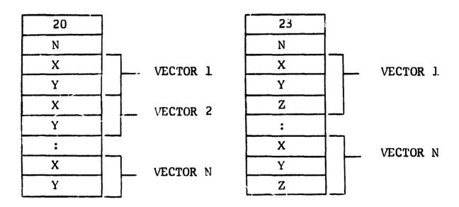
The range of X and Y after translation should be 0 to 1023. If a value is outside this range, the out-of-range edges are forced to the nearest edge (0 to 1023).
