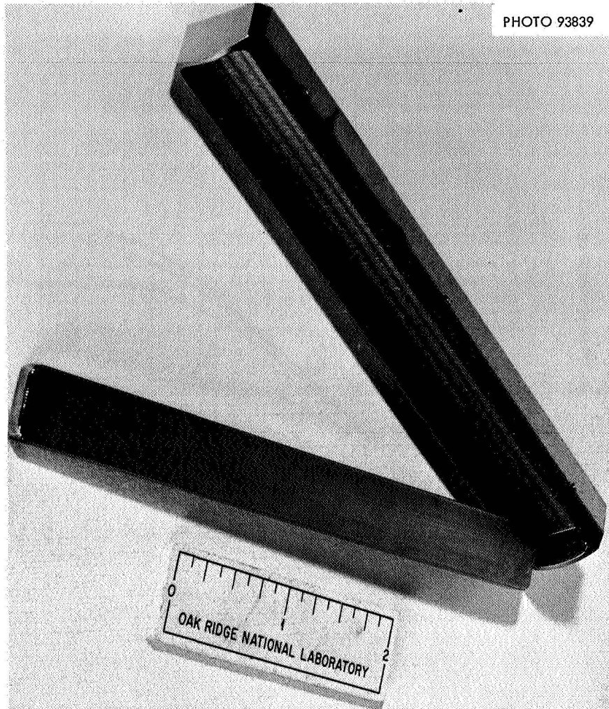
Fig. 6. Flat Plate ^{153}\text{Gd} Source and Shield.
