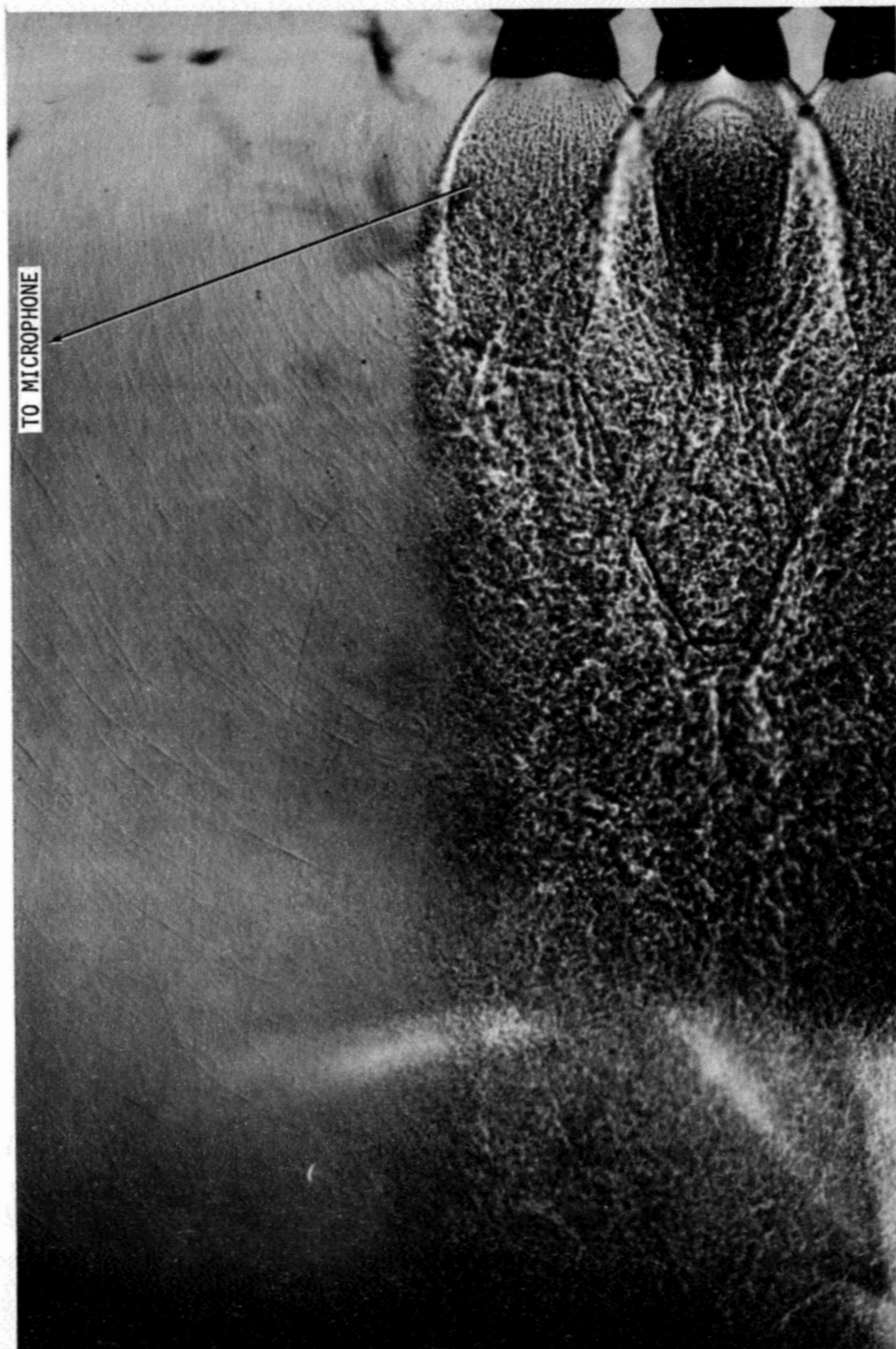
Figure 4-12. SHADOWGRAPH SHOWING MACH WAVE PATTERN AND MICROPHONE LOCATION
