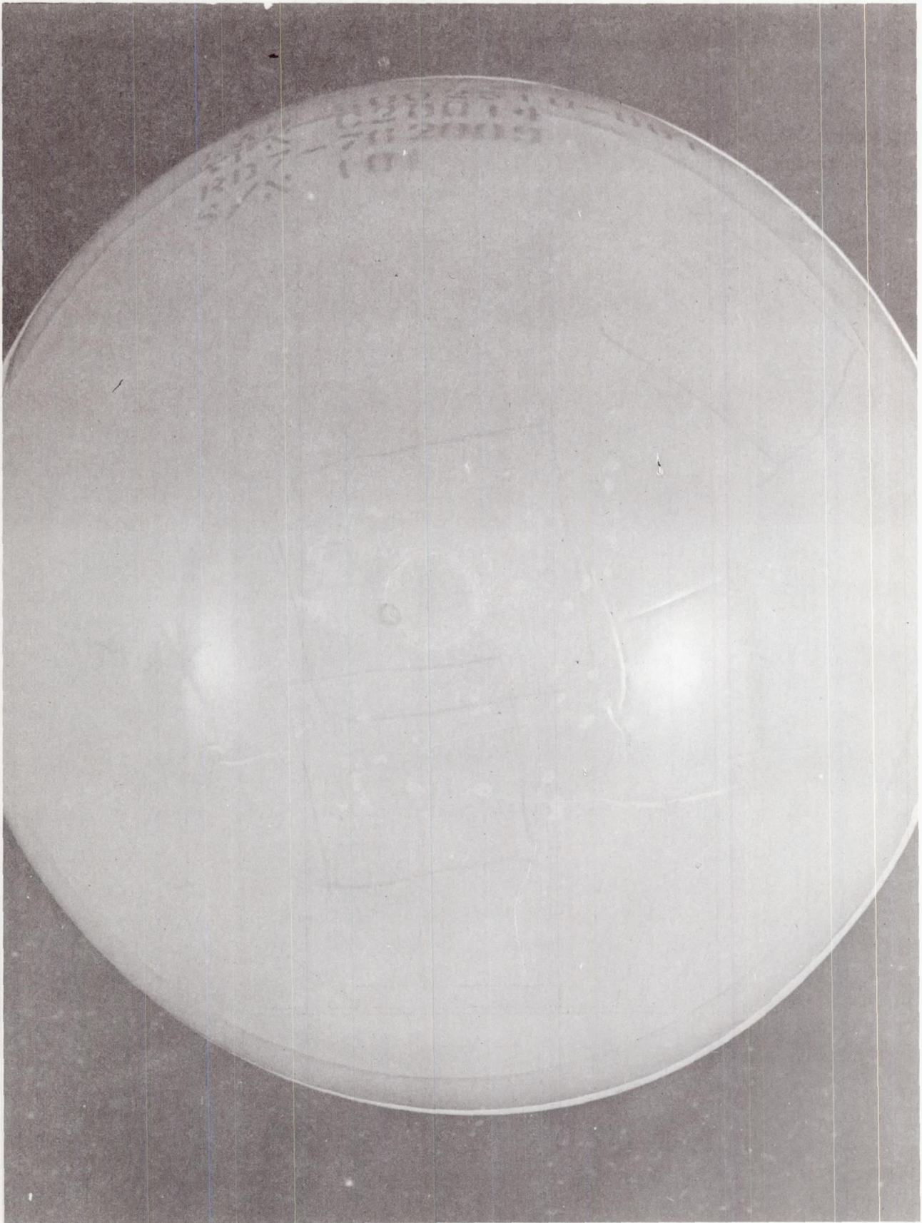
Fig. V-16 Oxidizer Tank Diaphragm
