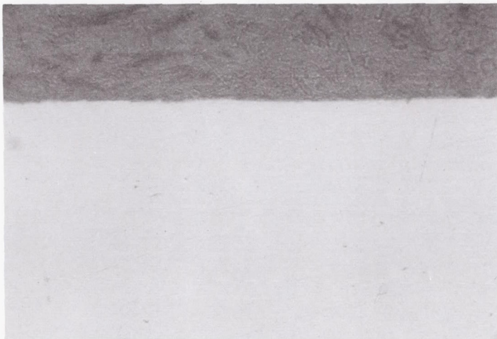
(a) Unnotched Specimen, Titanium 6Al-4V (200X)
