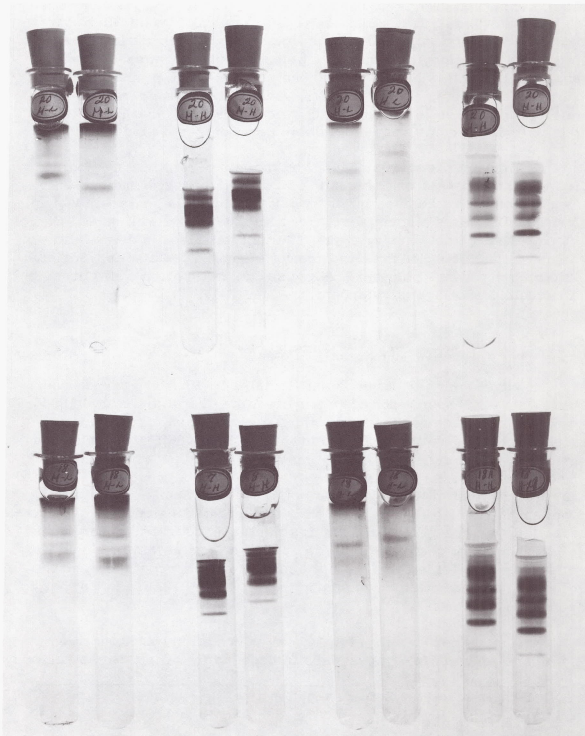
Figure 2. Photographs of Disc Electrophoresis Patterns of Mouse Muscle (M) or Heart (H) Extracts Resolved under Low (L) (pH 5.4) or High (H) (pH 8.6) pH Conditions.
