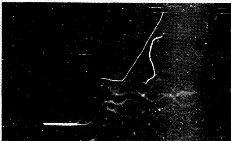
FIGURE D-3 DETECTOR OUTPUT (NO BIAS) OCEAN RETURN NO AGG 6 PULSES N_o/N_r = 20 DB 0.5 V/CM 40 N SEC/CM
