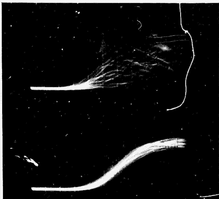
FIGURE D-5 DETECTOR OUTPUT OCEAN RETURN (TOP) N_o/N_r = 20 DB SINE WAVE SIGNAL (BOT) S/N_r = 16 DB AGC OPERATING DETECTOR BIASED 50 PULSES 0.1 V/CM 20 N SEC/CM
