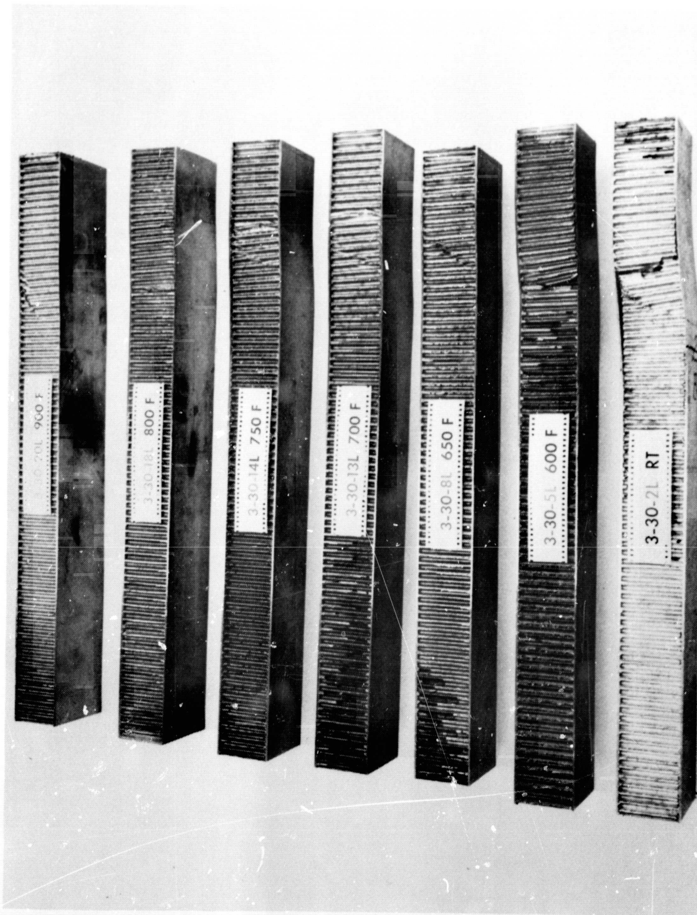
Figure 22.- Typical failures of 3-30 honeycomb core specimens (16.6 lb/cu ft) - longitudinal ribbon direction, each test temperature.
