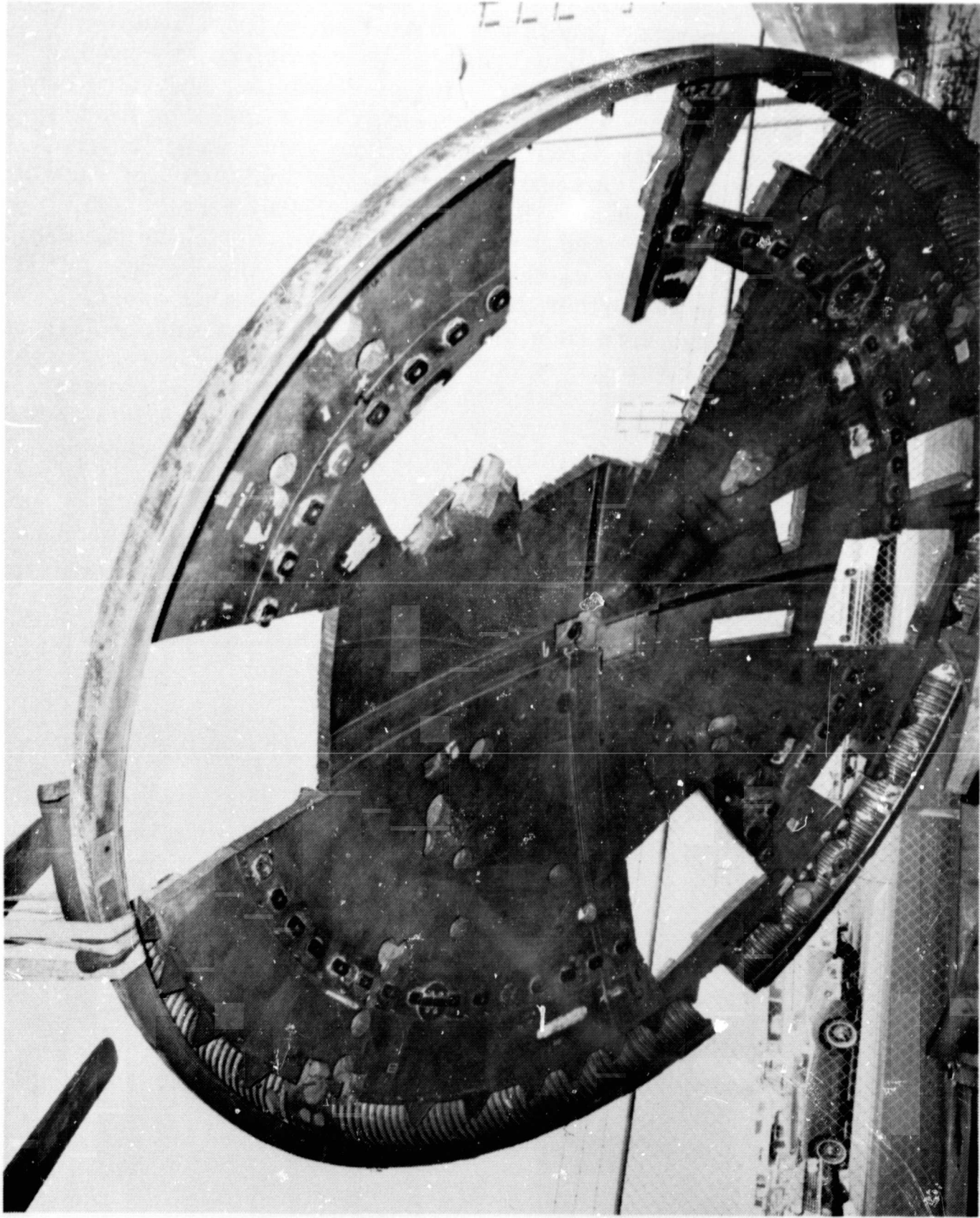
Figure 4.- Apollo heat shield (spacecraft 0i1) before specimen removal - inside view.
