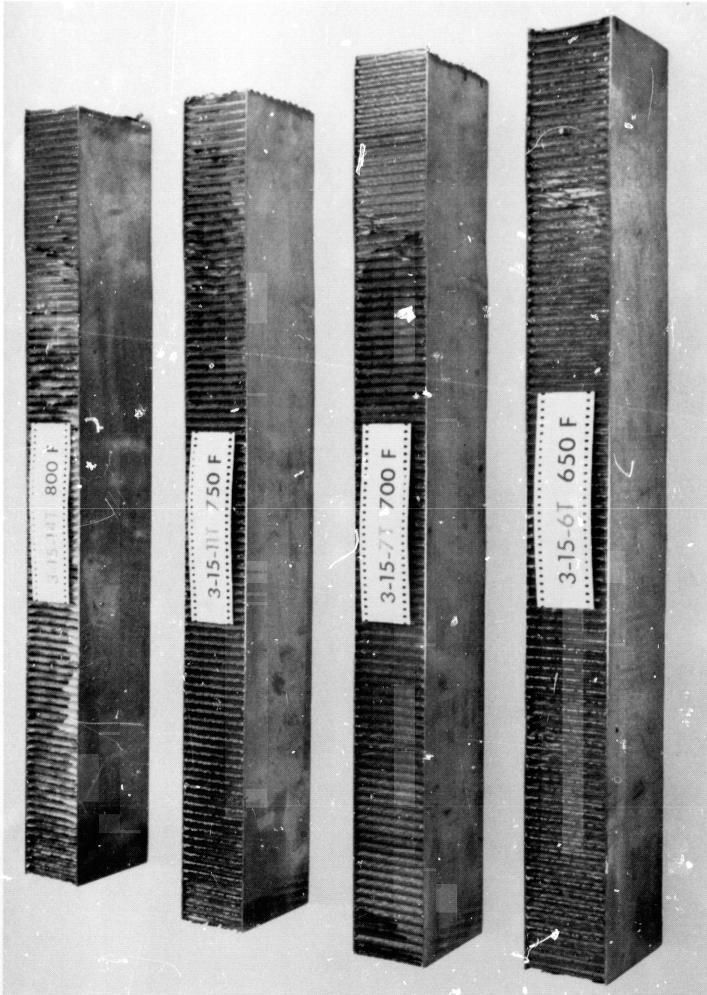
Figure 27.- Typical failures of 3-15 honeycomb core specimens (8.3 lb/cu ft) - transverse ribbon direction, each test temperature.
