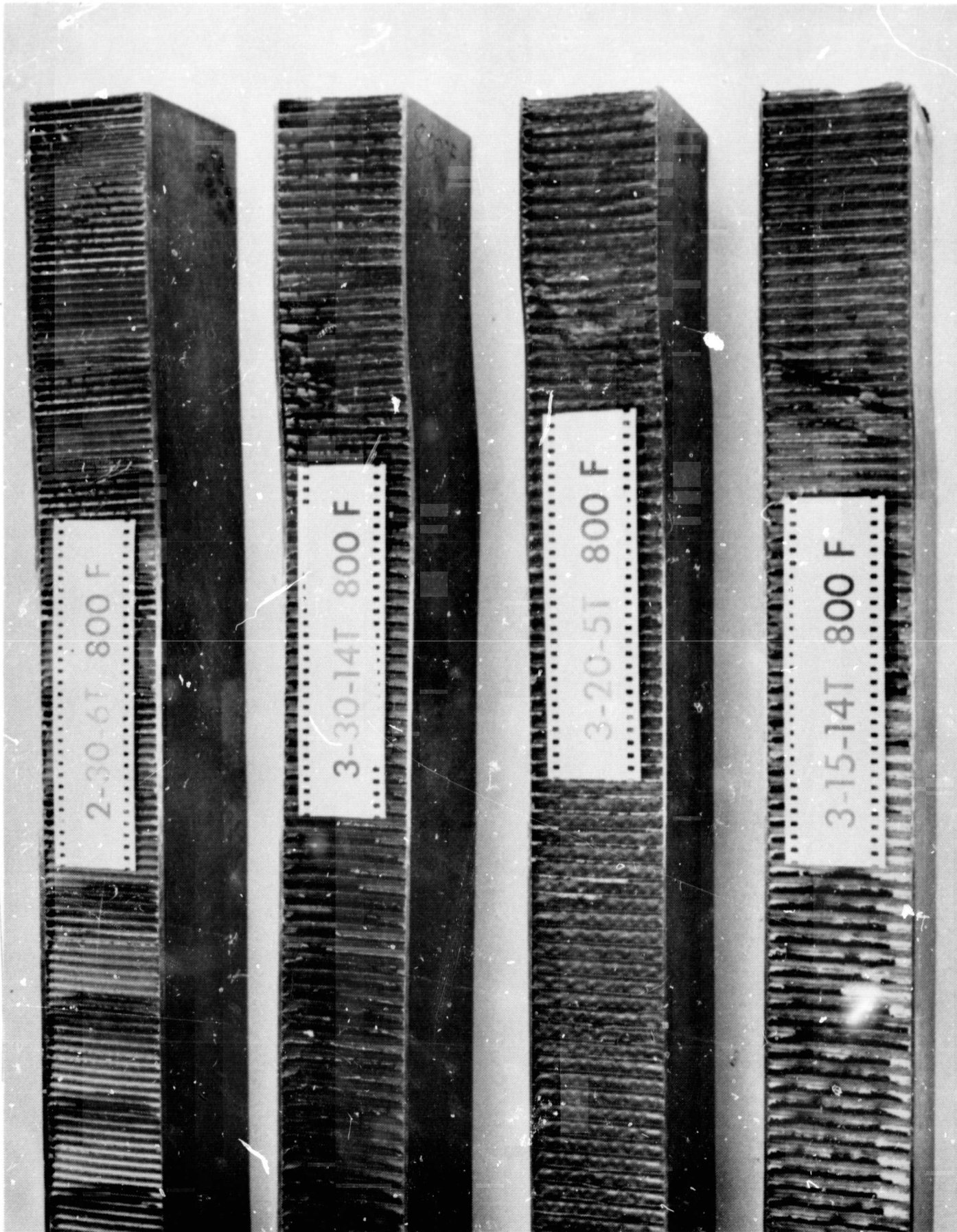
Figure 29.- Closeup of typical core shear failures.
