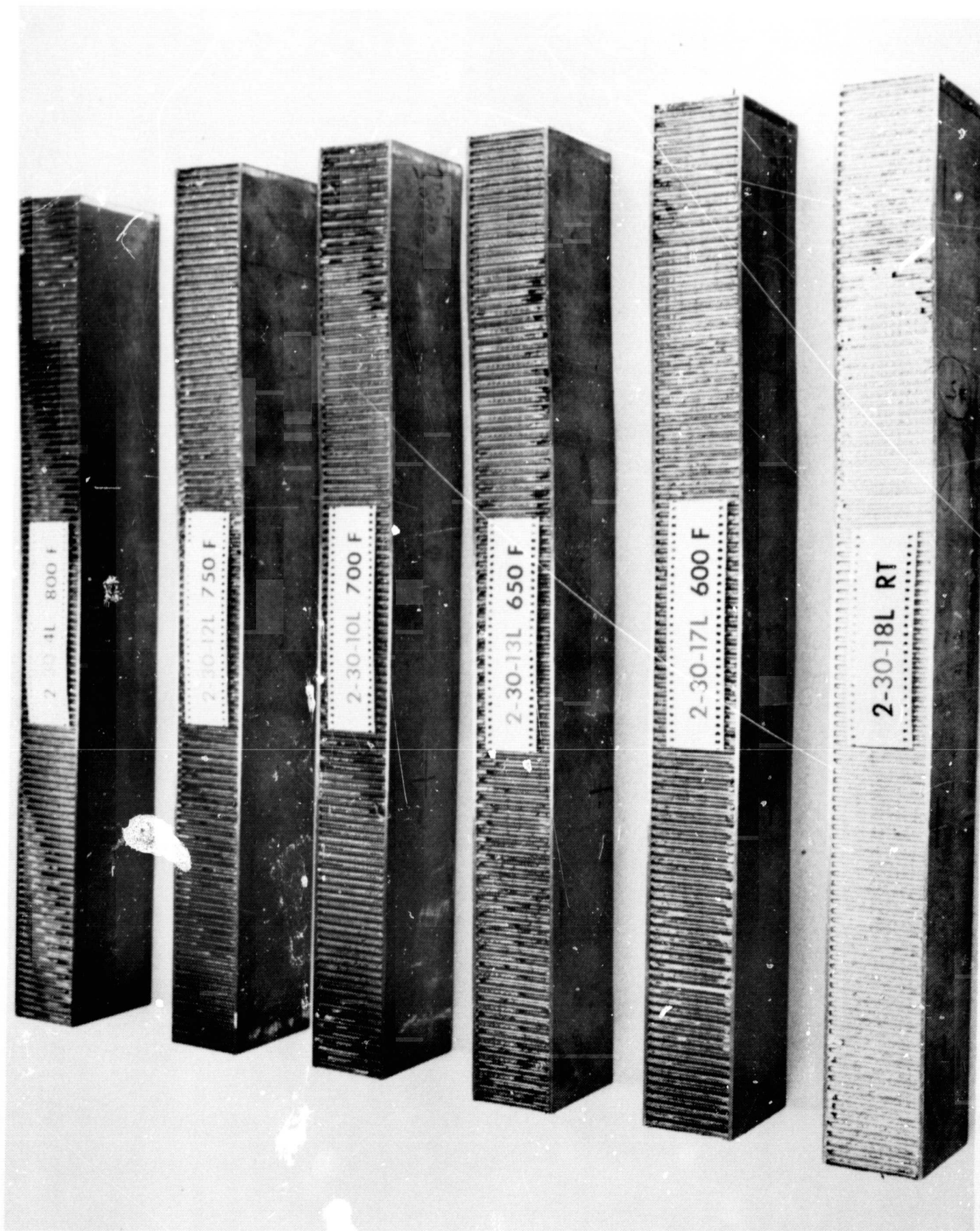
Figure 20.- Typical failures of 2-30 honeycomb core specimens (24.9 lb/cu ft) - longitudinal ribbon direction, each test temperature.
